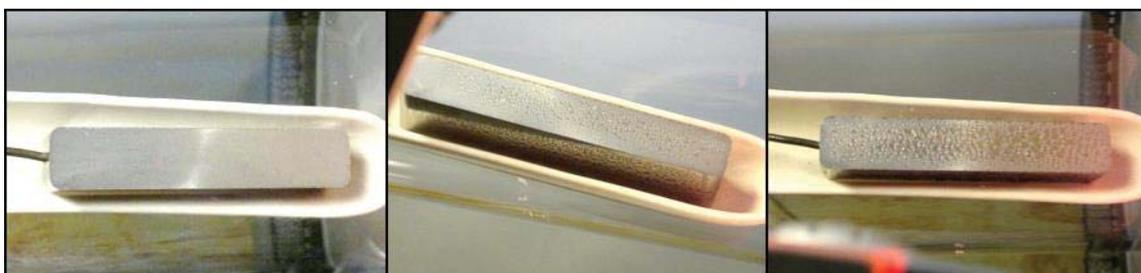
Figure 4 Images of the compact at different times during the delubrication process: visual observations from the present work
