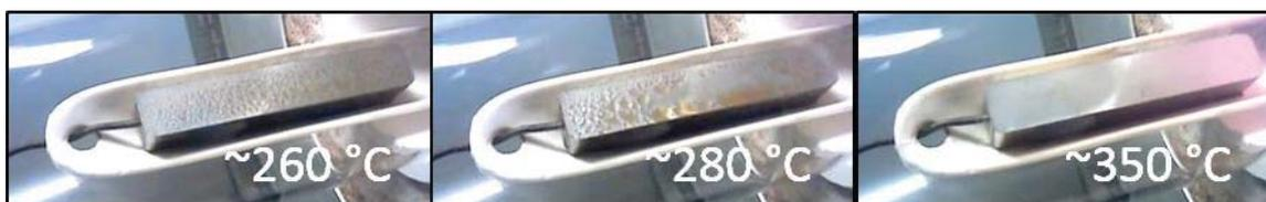
**Figure 20** Screen-shots from the video taken during different stages of delubrication of the sample
