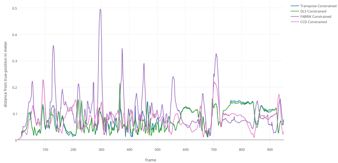
Figure 4.7: Distance to the true position of the knee when constraints were incorporated. Tested on a dancing sequence with the position of the knee joint removed.
