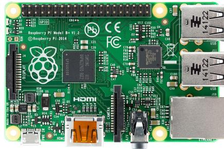
**Figure 7.1:** The Raspberry Pi single-board computer. Photo courtesy of Lucasbosch. [16]
