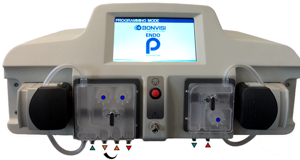
Figure 3.1: ENDO P® front view. Tubing ports on the cassettes are marked with arrows. Pressure sensors locations are marked with blue circles.
