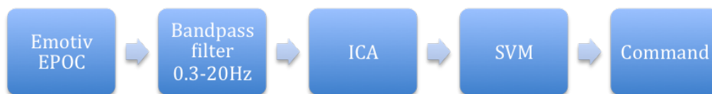
Figure 43: A overview of a BCI with the components established in this investigation inserted. This can be related to Figure 2 where the spatial filter inserted is the ICA and the classifier is SVM, also the used headset and digital filter properties are stated.
