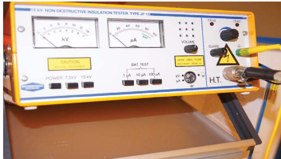
Figur 6: 15kV NON-DISTRUKTIVE INSULATION TESTER TYPE JP 15
