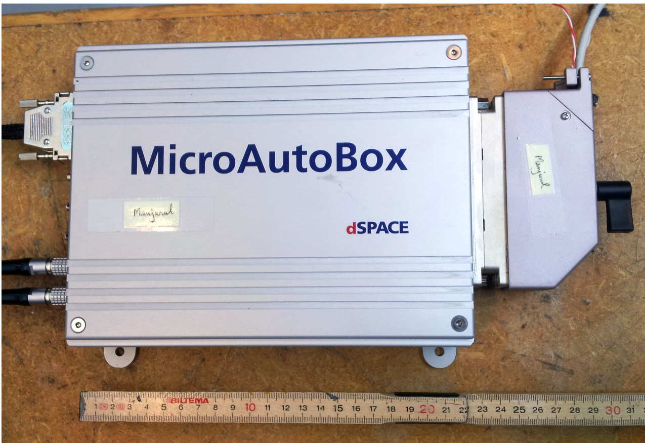
Figure A.3: dSpace MicroAutoBoxII viewed from the top including cables for ZIF-connector, Host-PC, Simulation-PC and power supply (clockwise, starting on the right)
