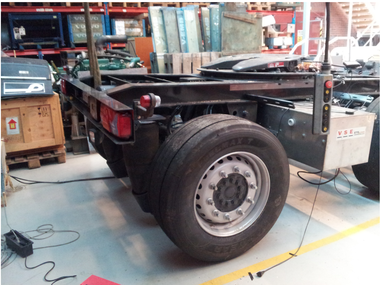
Figure A.2: Dolly craned up slightly to determine delay of steering actuation
