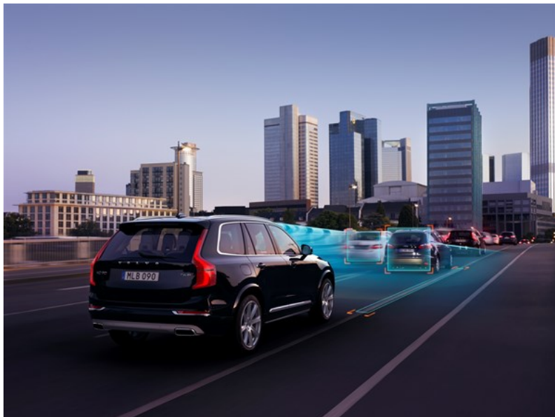
Figure 2.1: A Volvo XC90 using sensor and robot functions to follow a queue, Queue Support. Photo taken by Volvo Cars
