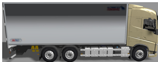
Figure 2.6: A Volvo truck from PreScan with a 6x2 axle setup. Photo from PreScan
