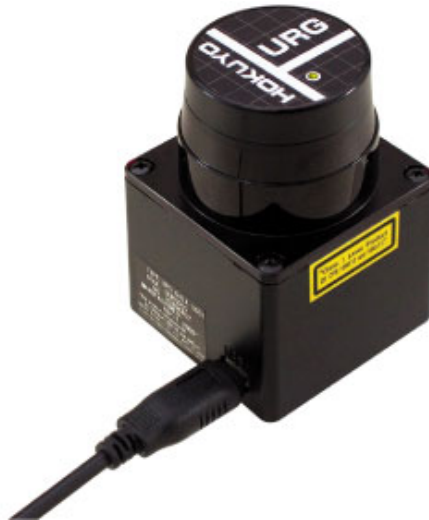
Figur 2.3: LiDAR, Hokuyo modell URG-04LX-UG01 [36]
