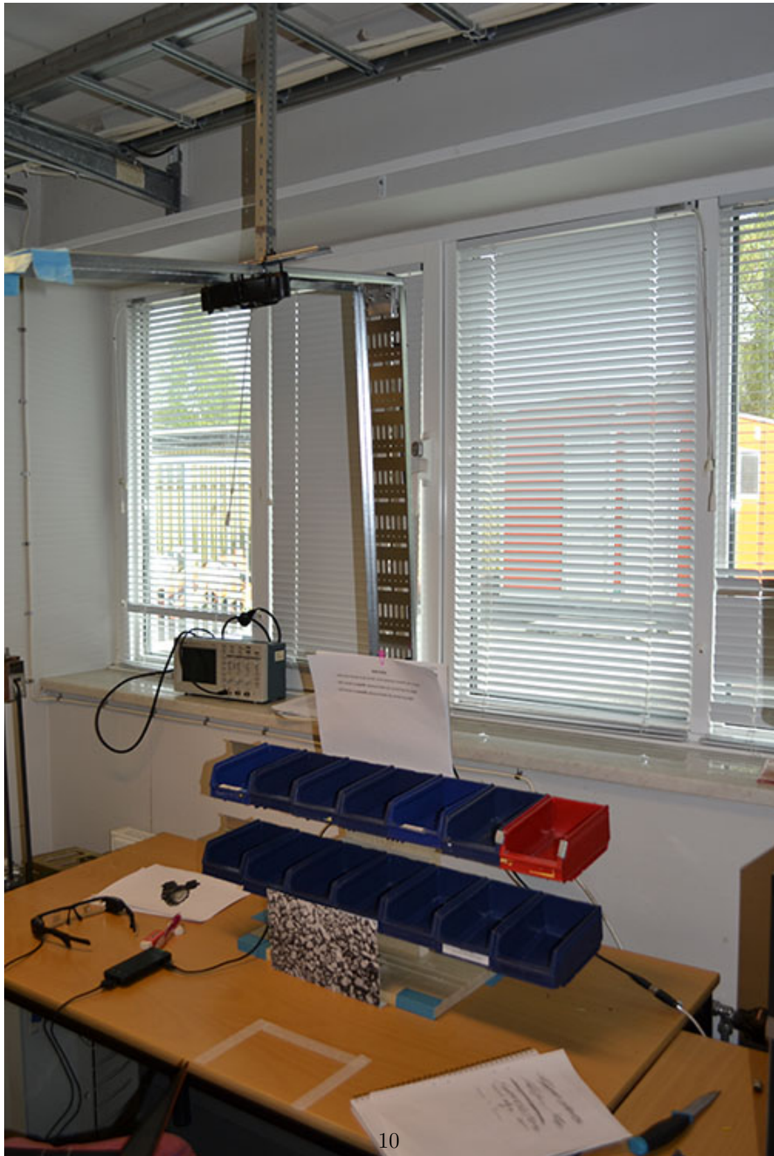
Figure 3.1: The experimental platform showing the 3D-camera, part boxes and the AR-glasses with the accompanying touchpad
