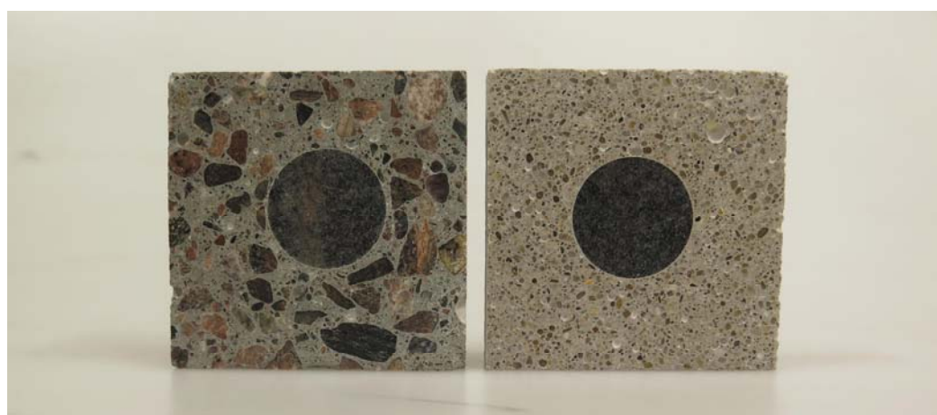
Figure 4.3 The two different types of concrete specimens; one with coarse cement mortar and one with fine cement mortar.
