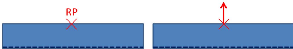
Figure 3.4 Boundary conditions for the upper part of the modelled specimen.
