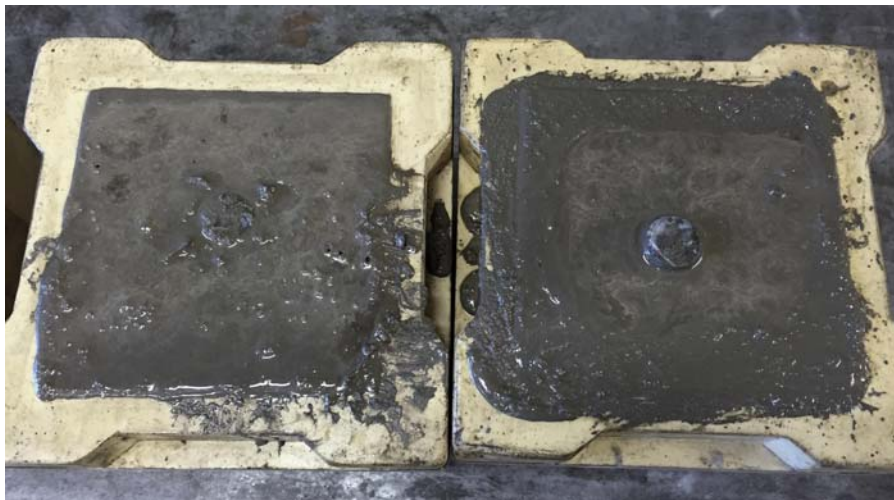
Figure 4.1 Casting of concrete blocks with a cylinder of rock material placed in the middle.
