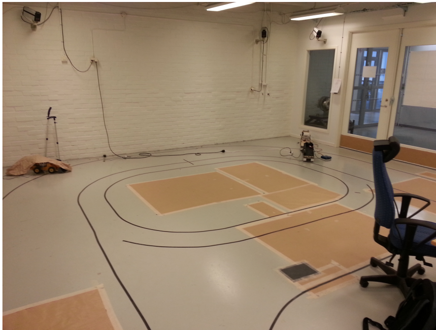
Figure 2.4: Photograph of IVRL, the laboratory where the testing was carried out. Some roads not used in this project are marked with tape on the ground, along with pieces of paper used to mitigate reflections. The LCV model is visible in the corner of the room.
