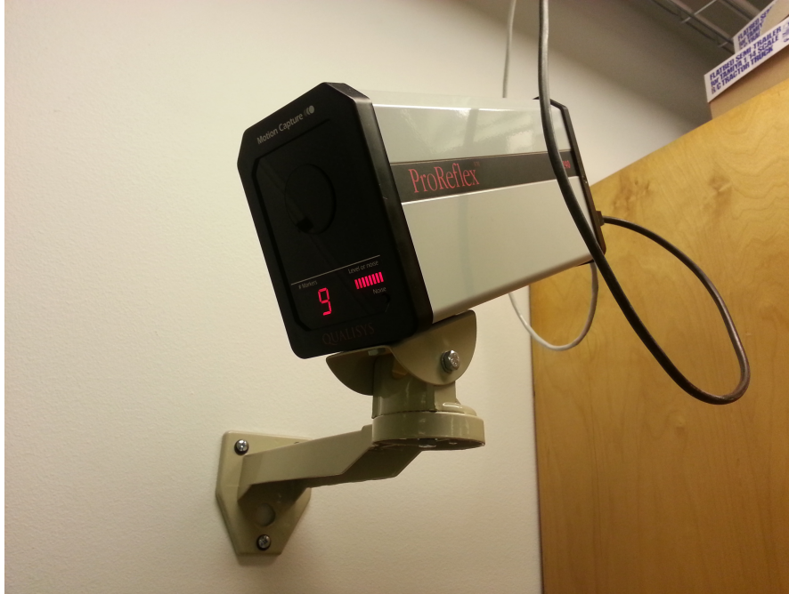
Figure 2.5: Photograph of a ProReflex camera by Qualisys, taken in the laboratory. Eight of these cameras were mounted on the walls in the lab, which made it possible to track objects in the room.
