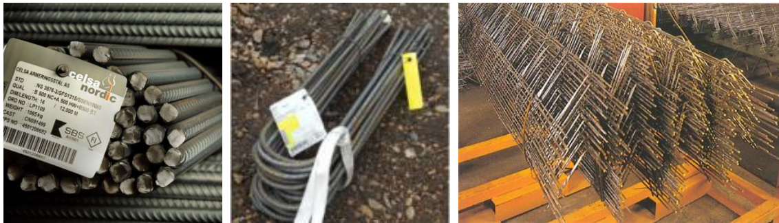
Figure 3 - Examples of rebar types. From left: Straight reinforcing bars, bent reinforcing bars, and welded reinforcing bars (Source: http://www.celsa-steelservice.se ).
