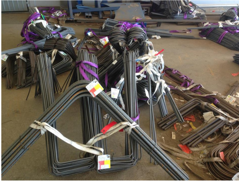
Figure 11 - Bent rebars at finished goods warehouse at Celsa.
