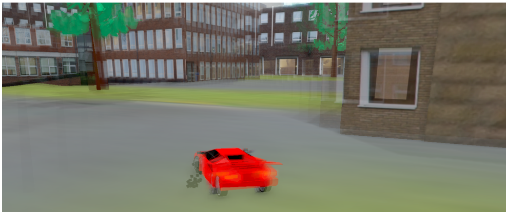
Figure 2.19: Edge detection-based motion blur sometimes become too aggressive.
