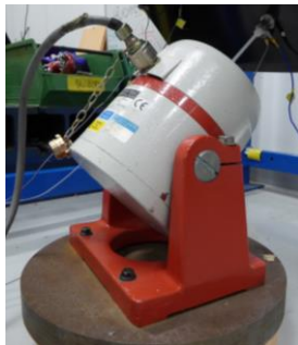
Figure 12: Shaker exciting the system. Brüel & Kjær LDS Ling Dynamic Systems Ltd. Model V406 – Permanent Magnet Shaker.
