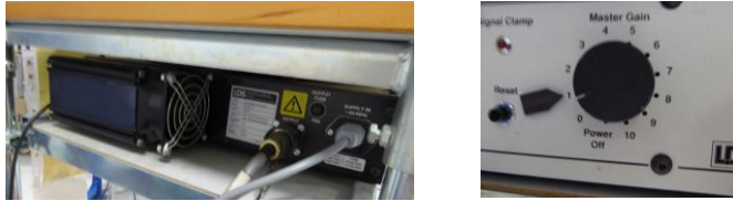
Figure 11: Amplifier of the excitation signal. Brüel & Kjær LDS Ling Dynamic Systems Ltd. PAE Series PA100E - Power Amplifier.
