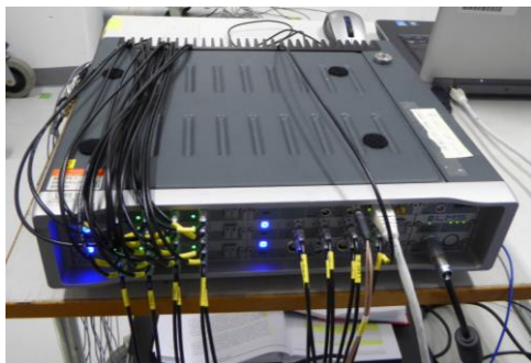
Figure 10: Frontend used in the measurement for data acquisition. LMS SCADAS Mobile SCR05. 40 channels, 2 outputs, 2 tachometers.
