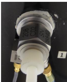
Figure 14: Force transducer to measure the input excitation. PCB Piezotronics Model 208C02 - ICP ® Force Sensor.
