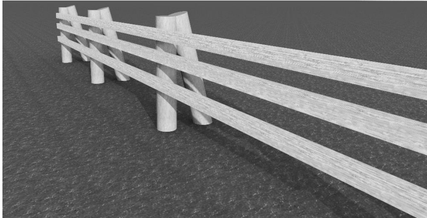
Figure 2.5 Simple protective piers made solely out of timber.
