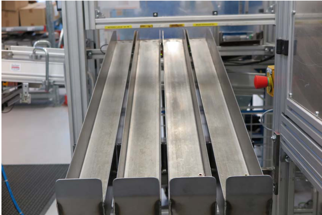
Figure 31. Escapement-tracks for different kinds of product defects.
