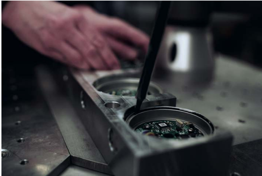
Figure 34. A pasting operation performed by a UR-robot.
