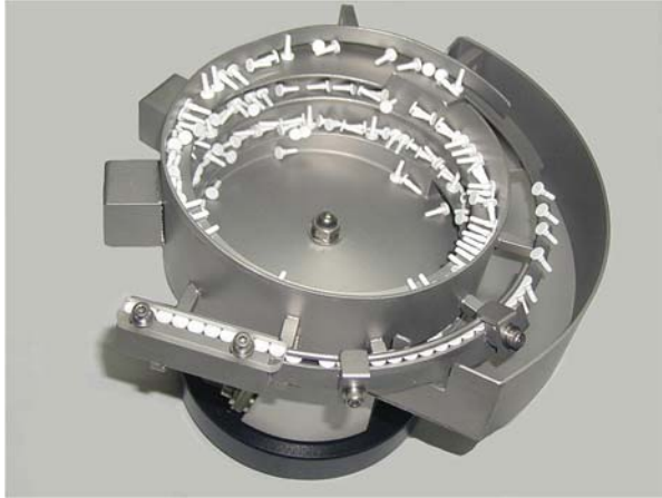
Figure 12. A typical vibratory-bowl feeder.
