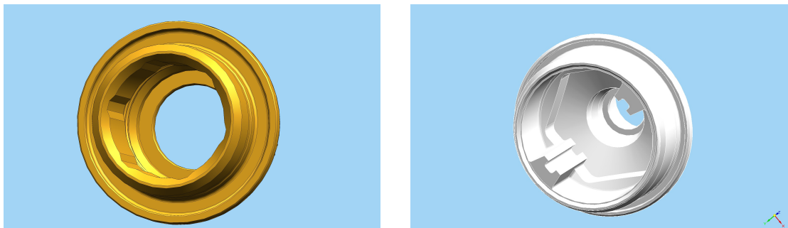
Figure 19 - Redesign of bonnet (left figure) compared to its original design (right figure)
