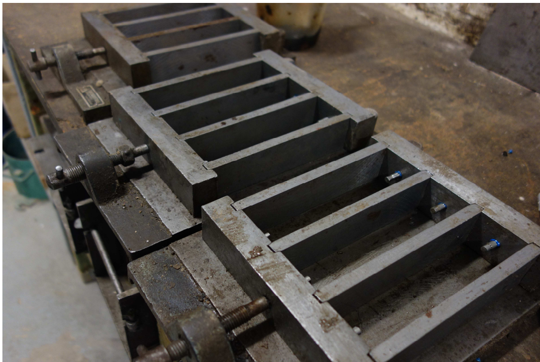
Figure 4.2 The molds, each for casting of three prisms of the sizes 160x40x40 mm 3 . (Photo: Sandra Bentland)
