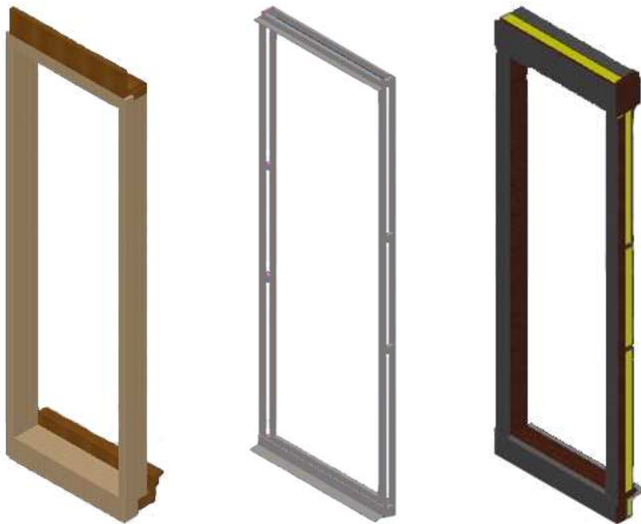
Figure 2.4 Left: The cross-laminated timber frame, here without galvanized steel covers. Middle: The load-bearing structure of the steel frame. Right: The steel frame equipped with insulation (in yellow), covering timber and galvanized steel covers.
