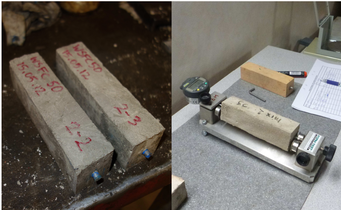
Figure 4.3 Left: The prisms after 48 hours of curing. The small steel bars were casted into the prisms so that they would fit into the measurement equipment. (Photo: Sandra Bentland) Right: The measurement equipment that tells the difference in length compared to the wood prism. (Photo: Helén Jansson)
