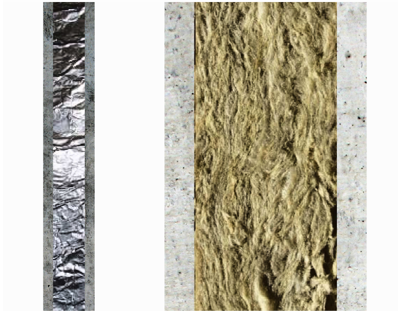
Figure 5.10 Illustration of the needed thickness of a sandwich element of vacuum insulation and textile reinforced green concrete (left) and a sandwich element of mineral wool and conventionally reinforced concrete (right) if a U-value of 0.10 \text{ W}/(\text{m}^2 \cdot \text{K}) is to be reached.
