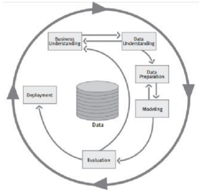
Figure 3 – Phases of the CRISP-DM reference model. (Chapman, et al., 1999)
