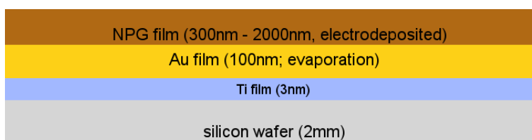
Figure 3.6: lateral Cu of Au electrode consisting of a silicon wafer as substrate, a 3nm Ti film, a 100 nm Au film form evaporation and a roughness factor dependent film thickness of NPG.
