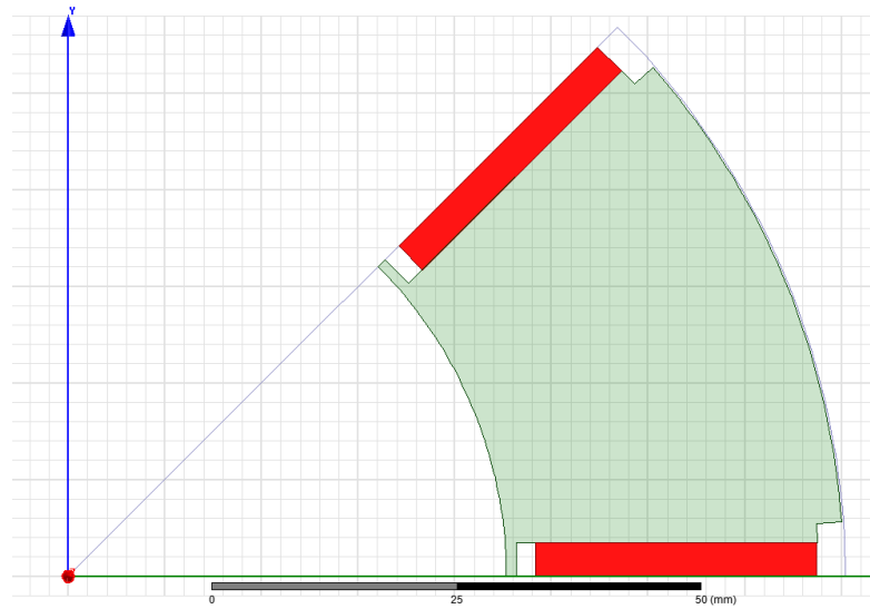
Figure 5.26: Rotor Geometry for Second Spoke Magnet Design.
