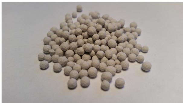
**Figure 2.5:** ZnO pellets from PowerCell
