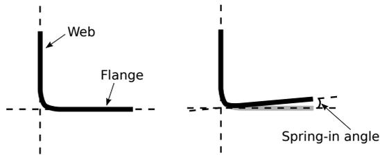
Figure 3.2: The spring-in phenomenon shown on an L-beam.
