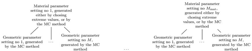
Figure 5.1: Variation simulation in two levels.
