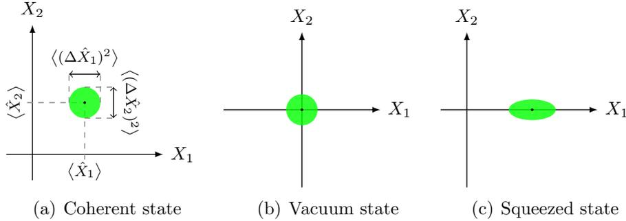
Figure 2.3: Phasor plots of various quantum mechanical states.
