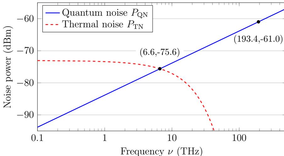
Figure 2.2: Comparison of quantum noise power  $P_{\text{QN}}$  and thermal noise power  $P_{\text{TN}}$  at a temperature  $T = 290$  K and with a detector bandwidth  $B_0 = 12.5$  GHz.
