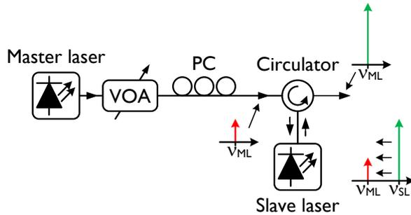
Figure 4.3: Illustration of setup for IL of laser.
