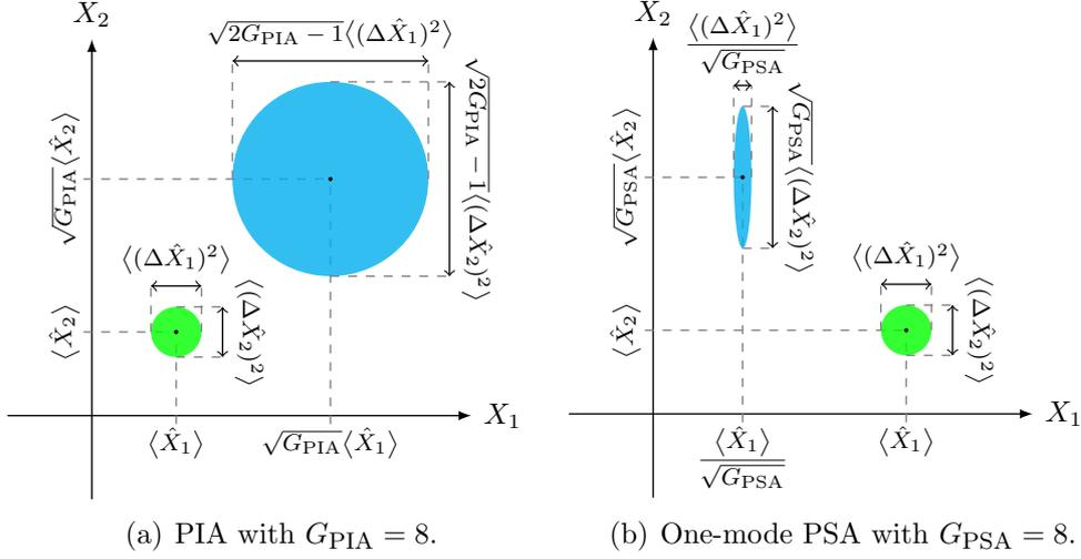
Figure 2.4: Illustrating of amplification of a coherent state using (a) a PIA and (b) a one-mode PSA. The input signal is illustrated by a green area and then output signal is illustrated by a cyan area.
