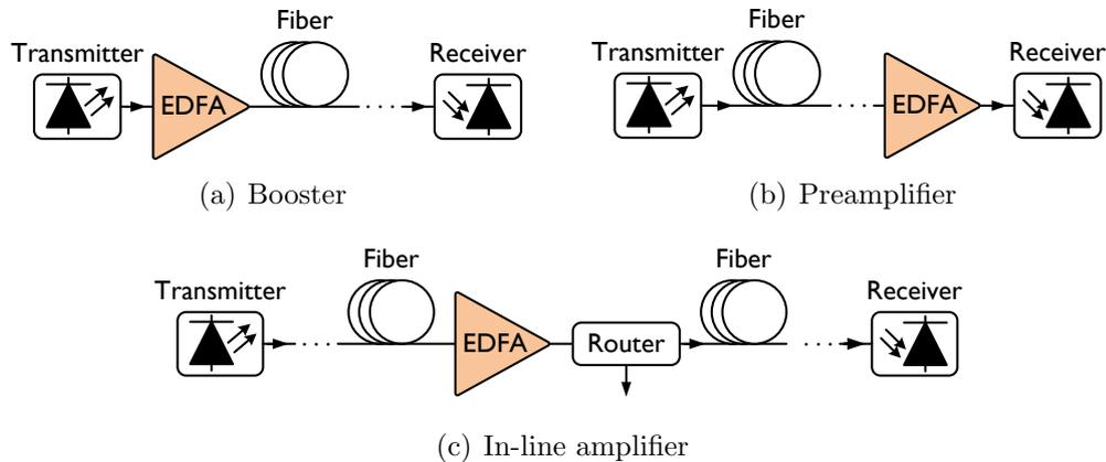
Figure 2.1: Illustration of possible amplifier placements.
