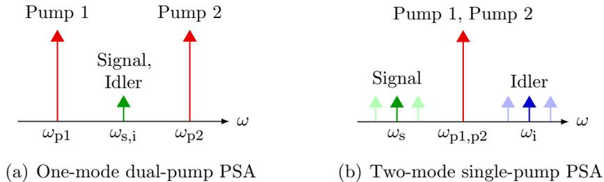
Figure 1.2: Examples of PSAs implemented using FOPAs.
