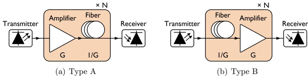
Figure 2.5: Illustration of possible in-line amplifier configurations.
