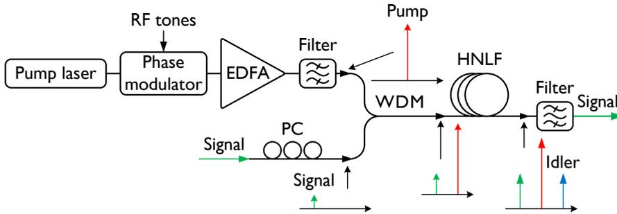
Figure 3.3: Typical implementation of a phase-insensitive FOPA with phase-modulated pump for SBS suppression.
