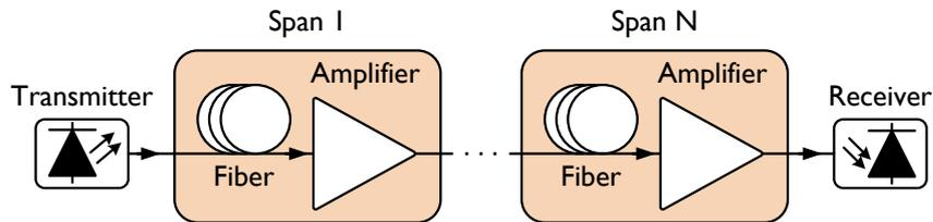
Figure 1.1: Illustration of a long-haul fiber optical communication system.
