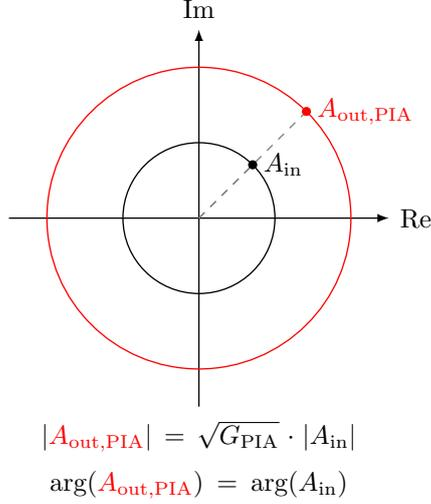
Figure 1.3: Illustration of input (black) and output (red) signals for a PIA with gain  $G_{\text{PIA}} = 4$ .
