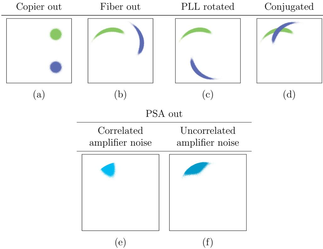
Figure 4.5: Step-by-step illustration of NLPN mitigation using a two-mode PSA-amplified transmission system with signal  $A_s$  (green), idler  $A_i$  (blue), and output (cyan).
