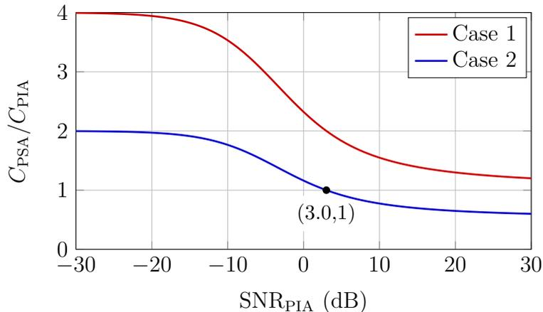
Figure 4.4: Comparison of two-mode PSA-amplified transmission systems to PIA-amplified transmission systems in terms of capacity. Transmission is assumed to be linear and benefits from nonlinearity mitigation are not considered.
