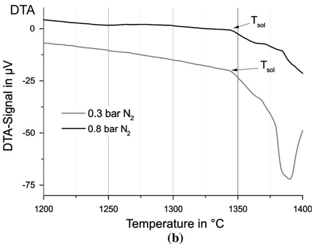
Fig. 2—(a) RGA-measurements revealing oxide reduction at  $\sim 1298$  K ( $\sim 1025$  °C) and  $\sim 1423$  K ( $\sim 1150$  °C) and (b) DTA measurements revealing a solidus temperature of  $\sim 1613$  K ( $\sim 1340$  °C) if nitrogen is applied as sintering atmosphere. Data is extracted from.<sup>[27]</sup>
