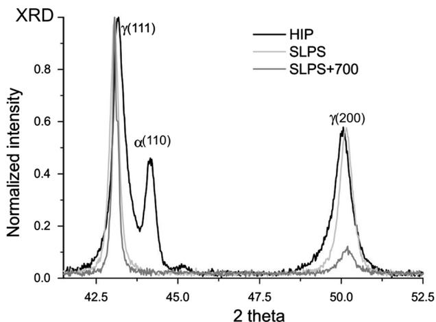
Fig. 9—XRD analysis of tested tensile specimens showing martensite formation ( $\alpha$ ) in the strengthened HIP specimen and a fully austenitic ( $\gamma$ ) microstructure of the strengthened SLPS-sintered specimens.
