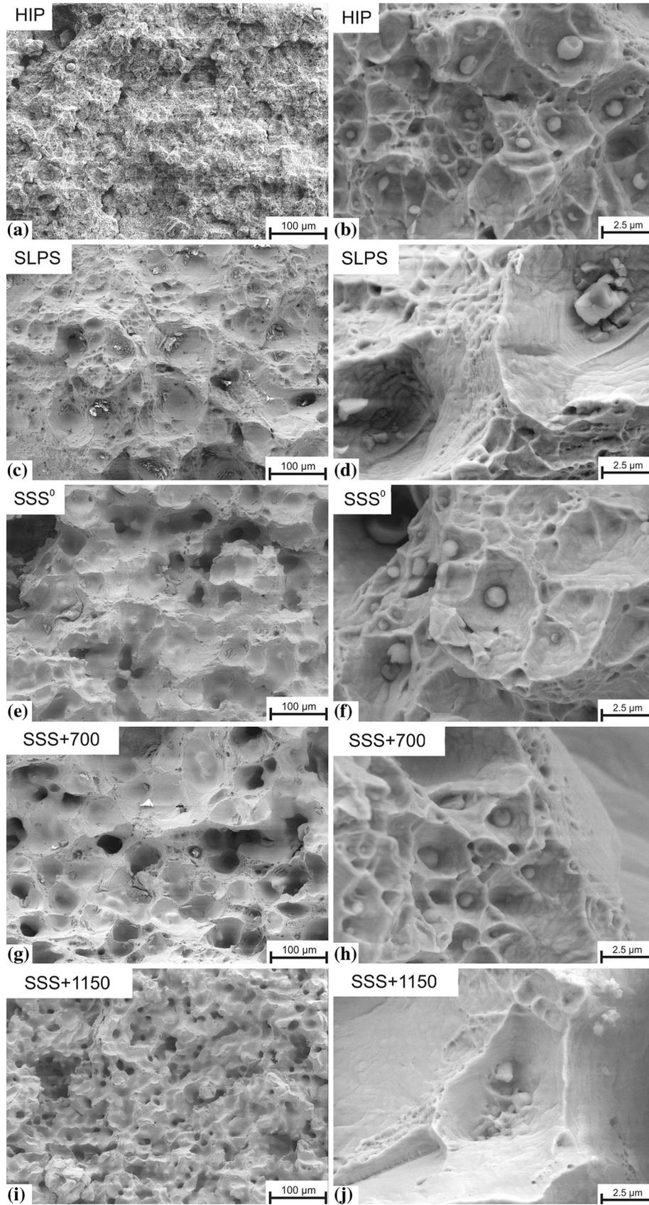
Fig. 5—SEM images of fractured surfaces of investigated specimens.
