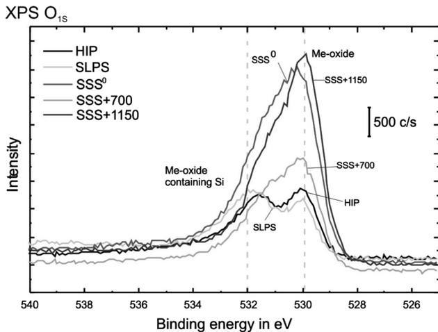
Fig. 4—Narrow scan of the  $O_{1s}$  oxygen peak of fracture surfaces revealing that specimens contain two types of oxides. The area under the graphs can be correlated to the amount of oxygen at the fracture surface.
