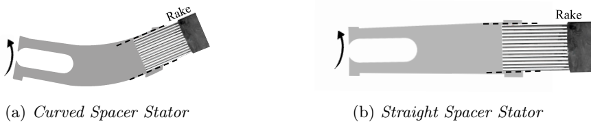
Figure 2.5: Alignment of Total Pressure Rake During Measurements
