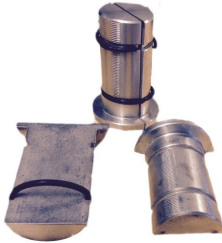
Figure 3.3 Custom made aluminium grips for Series 1.
