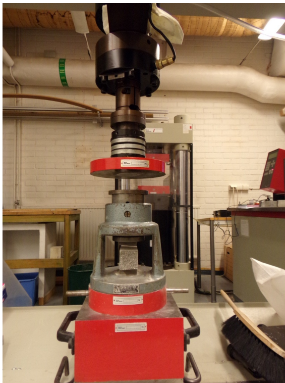
Figure 4.9 The compression machine for compressive strength test
