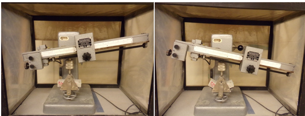
Fig. 4.7 The bending test machine for flexural strength
