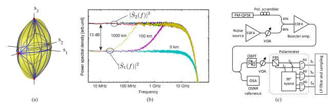
Fig. 1. (a) The Stokes representation of PM-QPSK. (b) The simulated spectrum of the Stokes parameters for different fiber lengths. (c) The experimental setup. VOA: Variable optical attenuator, OBPF: Optical band-pass filter, OSA: Optical spectrum analyzer, PBS: Polarization beam splitter, BD: Balanced detector, LP: Low-pass
