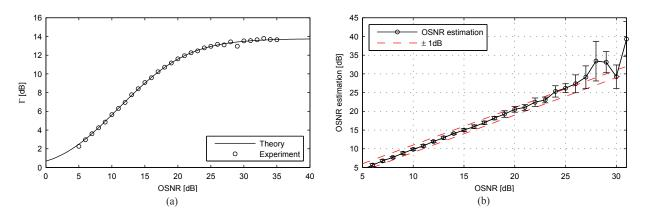
Fig. 2. (a) The theoretical curve for  $\Gamma$  together with experimental values. (b) OSNR estimation. The error bars represent the standard deviation of the dB-values of ten measurements.
