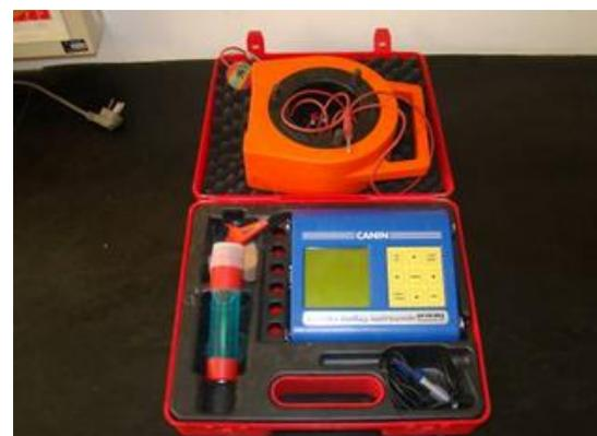
Figure 25 Reinforcement corrosion tester
