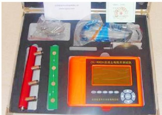
Figure 26 Resistivity tester for concrete resistivity measurement
