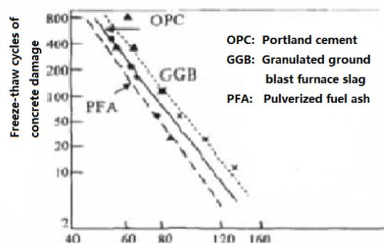
Figure 4 The relationship between water absorption ability of concrete and the resistance to freeze-thaw cycles (freeze-thaw cycles when concrete is damaged) (Liu, 2013).
