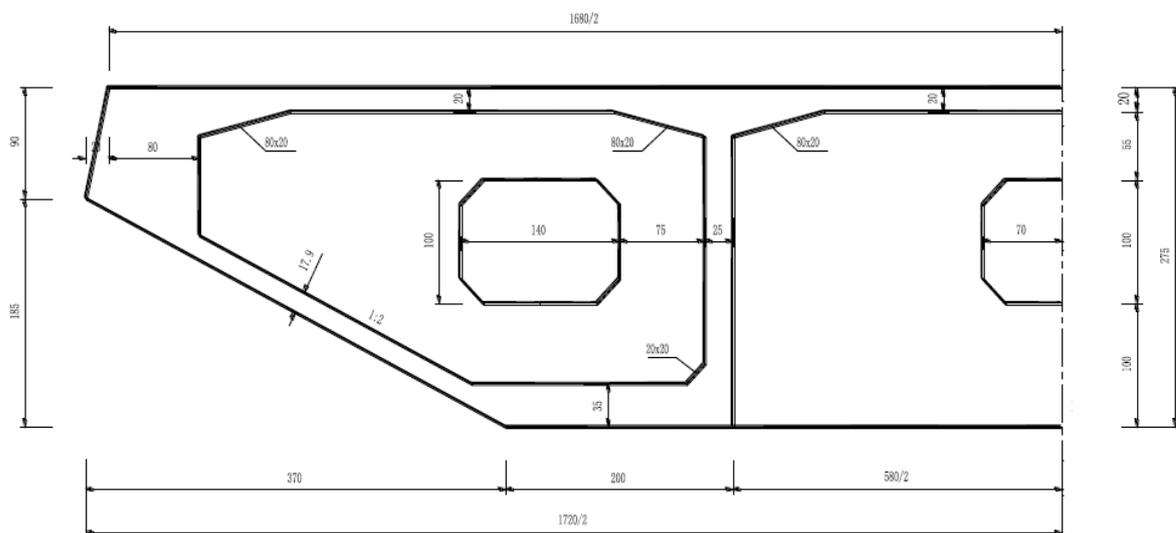
Figure 9 Every chamber is made up of roof, floor, straight web, inclined web, and diaphragm. There a manhole in the middle of the diaphragm.
