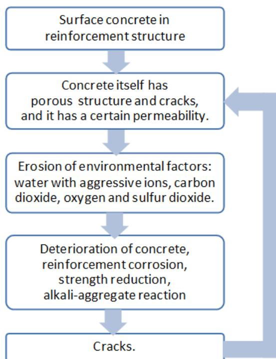
Figure 3 The deterioration process of reinforced concrete due to material properties and external environmental factors
