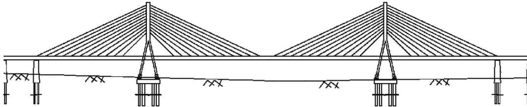
Figure 10 The cable-stayed bridge consists of two towers, eleven pairs of cables on each cable plane and the main girder (Song et al., 2007).
