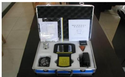
*Figure 20 Crack width gauge is used to measure the crack width*
