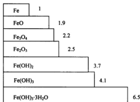
Figure 6 The volume expansion of the rust becomes greater when the degree of oxidation is higher (Deng, 2012).
