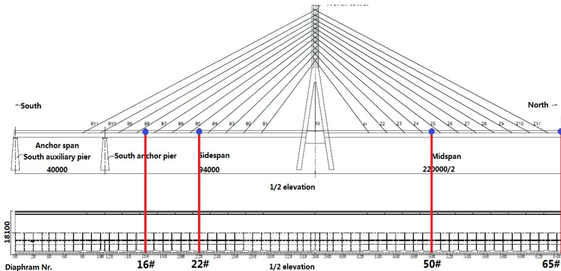
Figure 21 The location of four testing chambers
