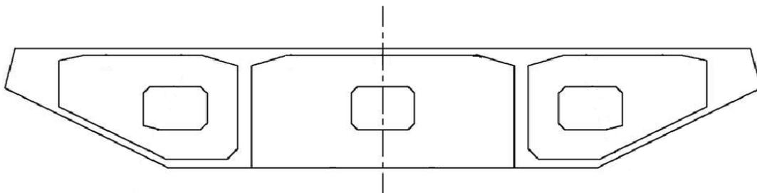
Figure 8 The main girder is a box girder. It has two closed chambers with trapezoidal shape.
