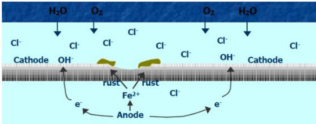
Figure 5 Chloride ion ingress occurs in the reinforced bars with the presence of oxygen and water. An electro-chemical cell is formed with the unprotected steels serving as the anode and the protected steel serving as the cathode. Rust is generated.
