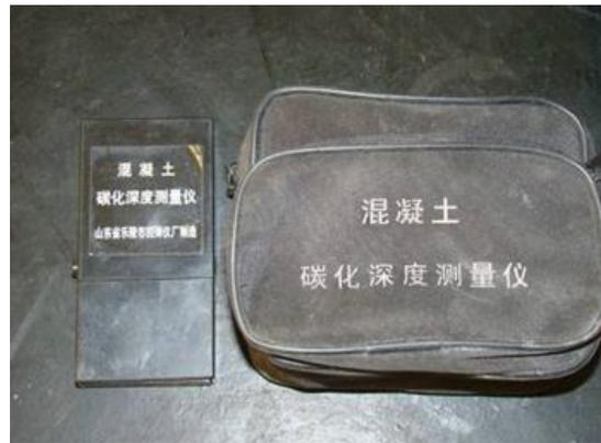
Figure 23 Phenolphthalein for concrete carbonation depth measurement
