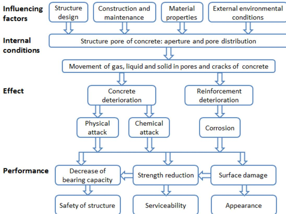
Figure 2 How the different factors influence the durability and the performance of reinforced concrete structures
