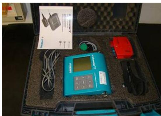
Figure 24 Reinforcement position and cover thickness measuring device
