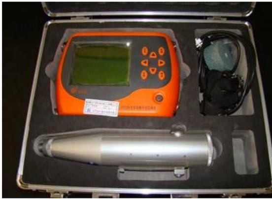
Figure 22 Resiliometer for concrete strength measurement
