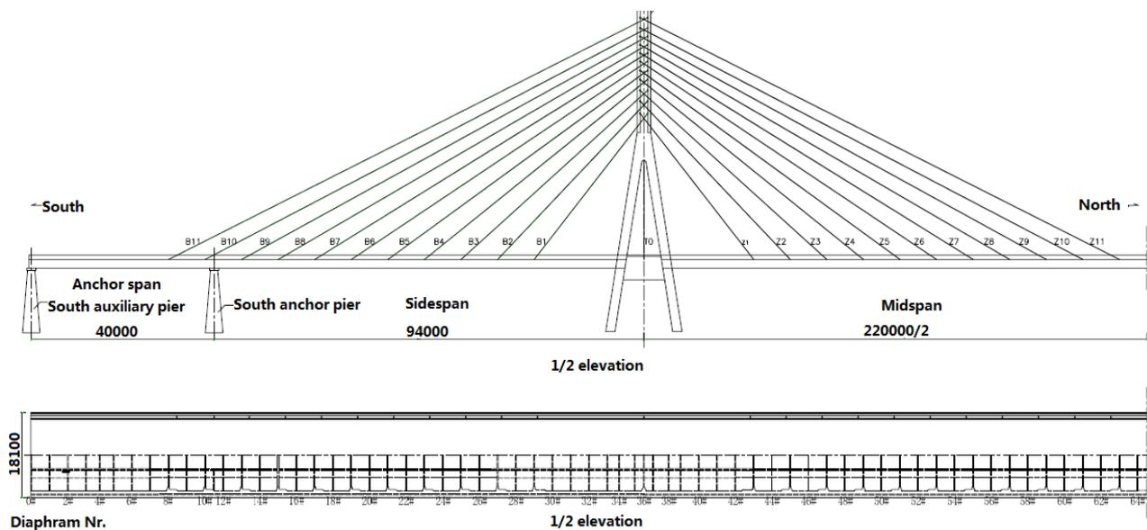
Figure 19 The number of the diaphragm starts from 0# to 65# from south to north. And the inspections start from diaphragm 11# at the south anchor pier to the diaphragm 65# at the middle of mid-span.
