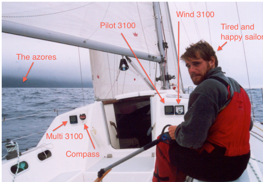
Figure 3.2: Picture of the cockpit of “Le RM 1050” with the speedometer/sound-meter, the autopilot, the electronic weathercock and the compass.
