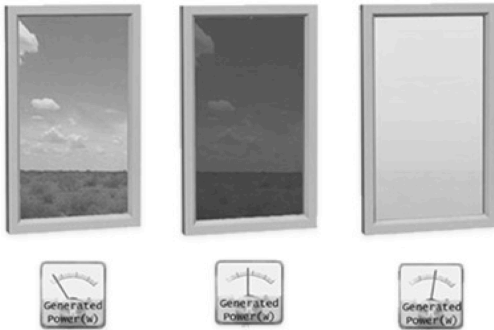
Figure 3.9 Different stages of the Smart energy glass and a principle indication of the generated electric power (PEER +)
