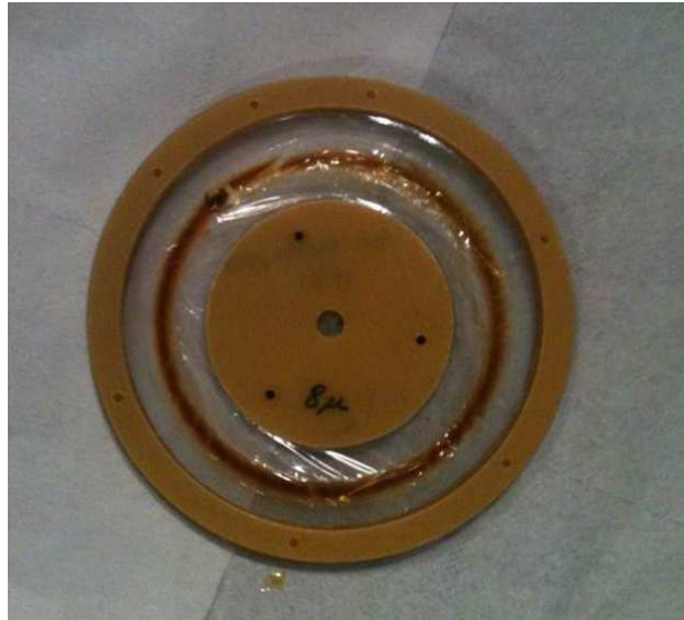
Fig. 3. Image of a stack of 8µm polypropylene targets after several days of irradiation at high beam currents.
