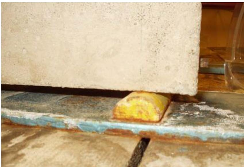
Figure 5.5 Support of the beam
