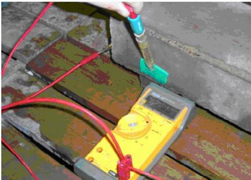
Figure 5.10 Half cell potential measurement
