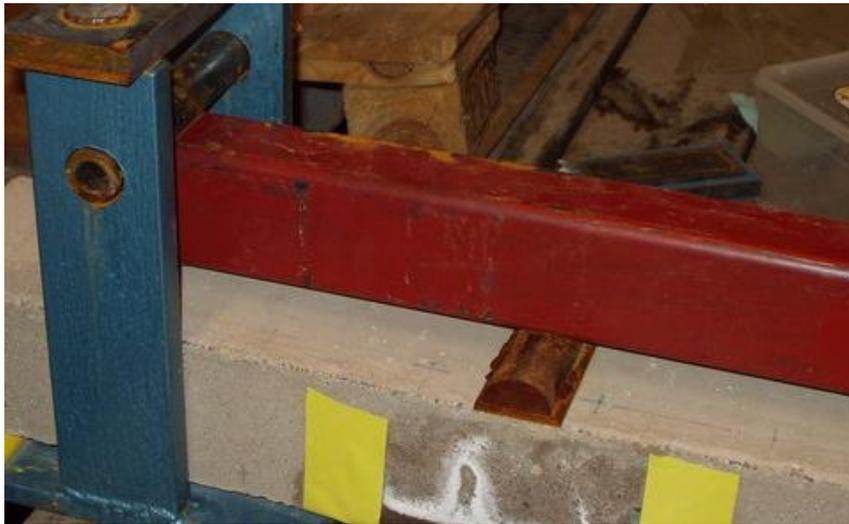
Figure 5.4 Load applied on the beam
