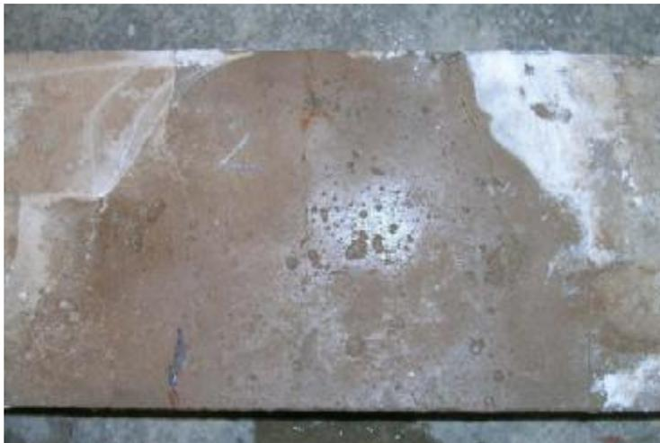
*Figure 5.11 Crack and rust products on the surface of a specimen*
