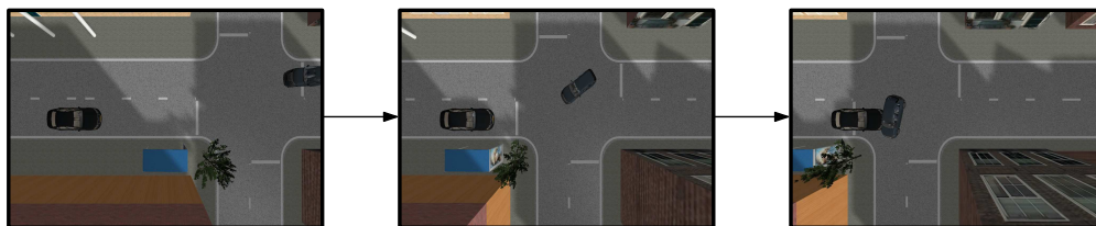
(a) A left turn across path performed by the other vehicle. Both vehicles had base speeds of 13 m/s.
