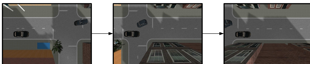
(b) A left turn across path is initiated by the other vehicle, but stops before entering the ego vehicles planned path. Both vehicles had base speeds of 13 m/s.
