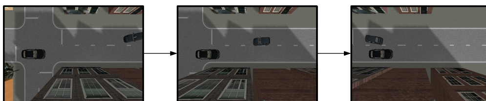
(c) The other vehicle avoids an obstacle in the opposing lane and then returns back to the centre of the lane. Both vehicles had base speeds of 13 m/s. This scenario has been used in the results presented in this section.
