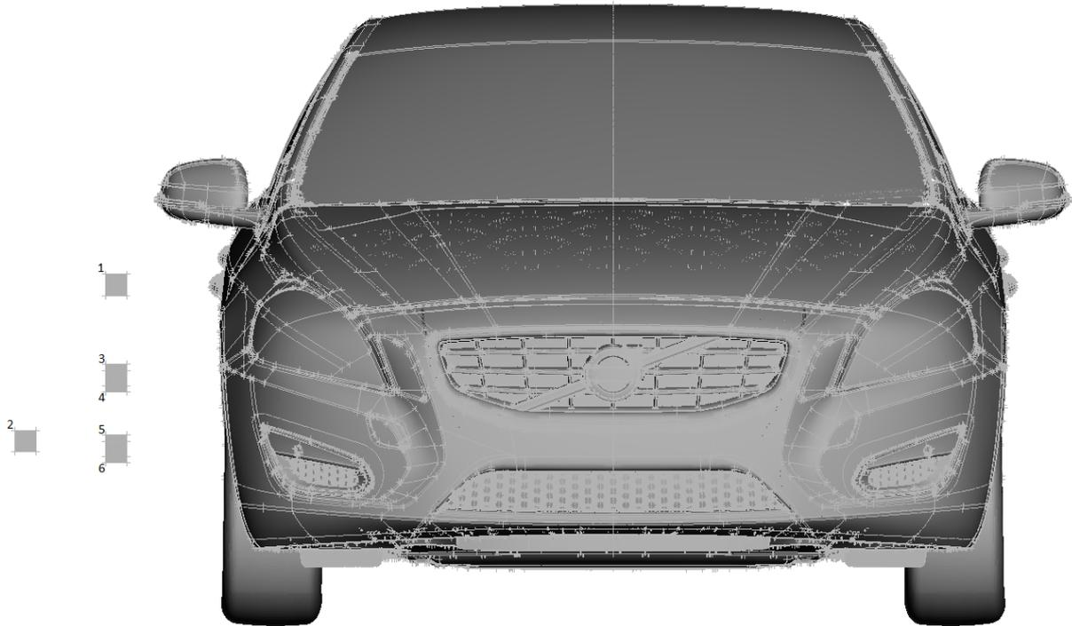
Figure 3.3: *The surfaces representing the locations of the precipitation sensor domains.*
