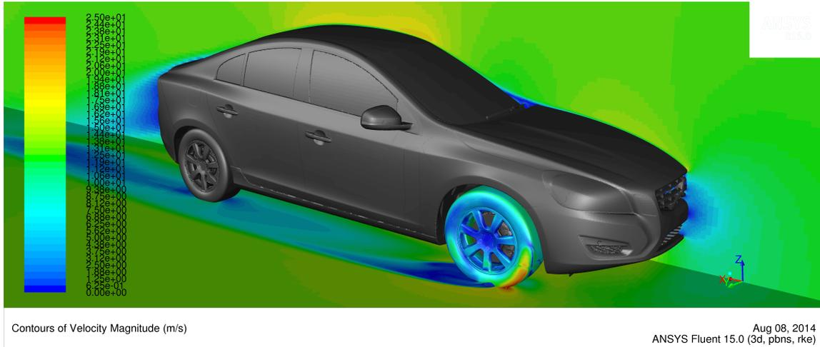
Figure 5.3: The velocity contours at different planes and surfaces over the car.
