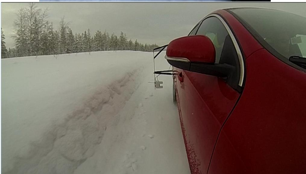
Figure 1.1: *The mounted sensor on the car. The height of the sensor can be adjusted to reach different locations. The flux distribution with respect to different locations are obtained in such manner. The test was done under VCC at Jokkmokk Proving Ground(JPG) around February, 2014.*
