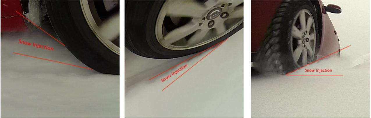
(a) *Snow particle injection, type 1.*      (b) *Snow particle injection, type 2.*      (c) *Snow particle injection, type 2.*
