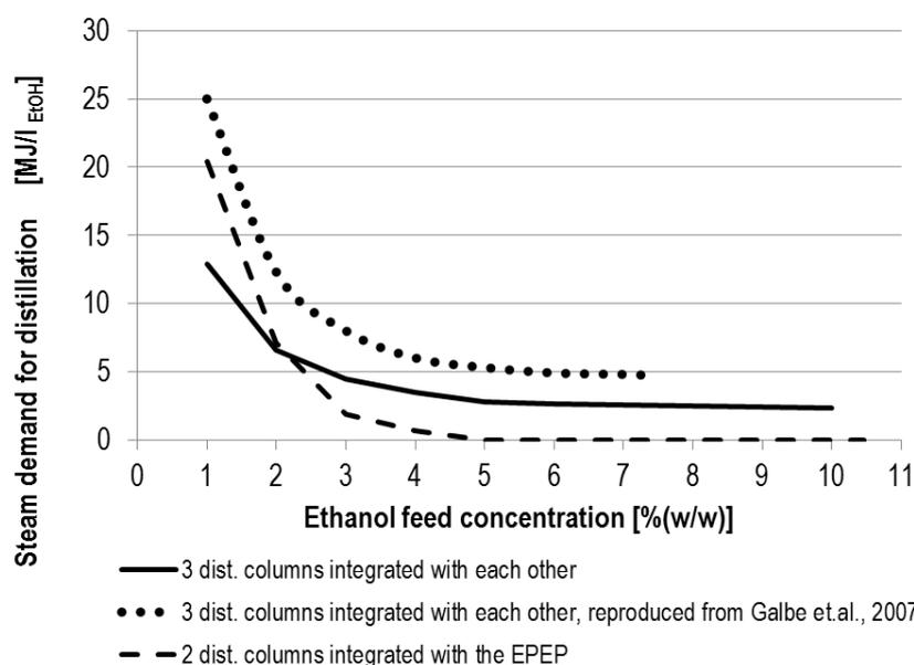
Figure 17 Resulting steam demand in the distillation plant.
