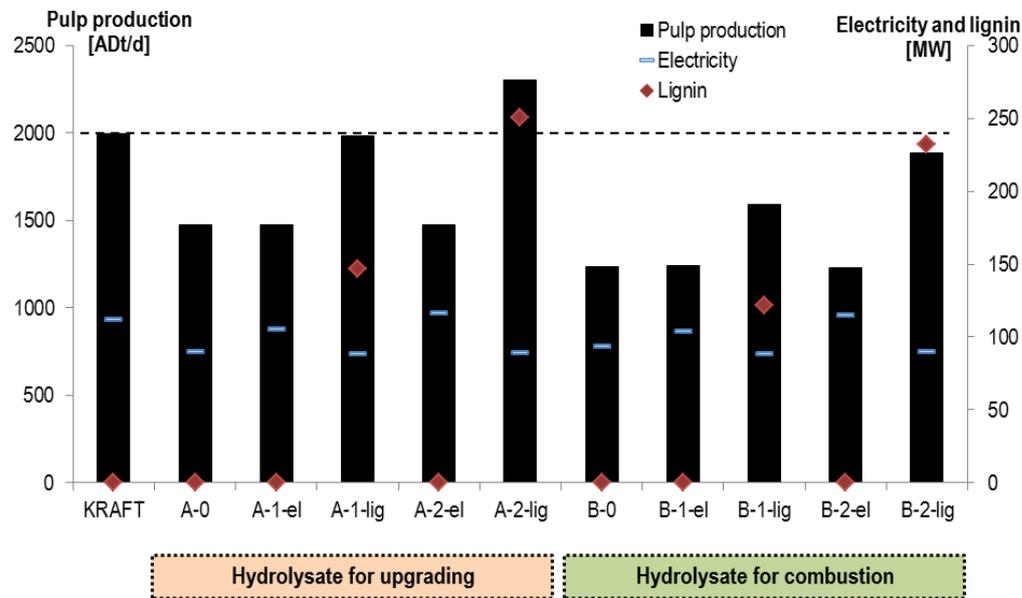
Figure 12 Pulp production capacity (left axis) and energy outputs (right axis) when the recovery boiler is the bottleneck for pulp production.
