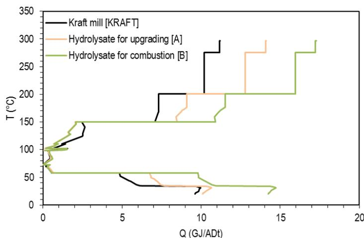
Figure 11 Grand composite curves for the kraft pulp mill, the dissolving pulp mill when the hydrolysate is sent to be upgraded and the dissolving pulp mill when the hydrolysate is burned in the recovery boiler.
