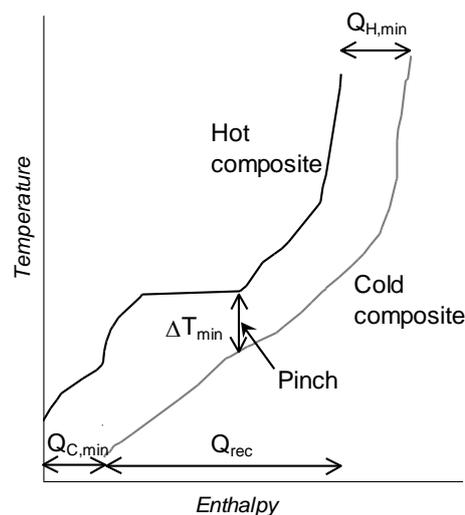
Figure A1: Example of Composite Curves.
