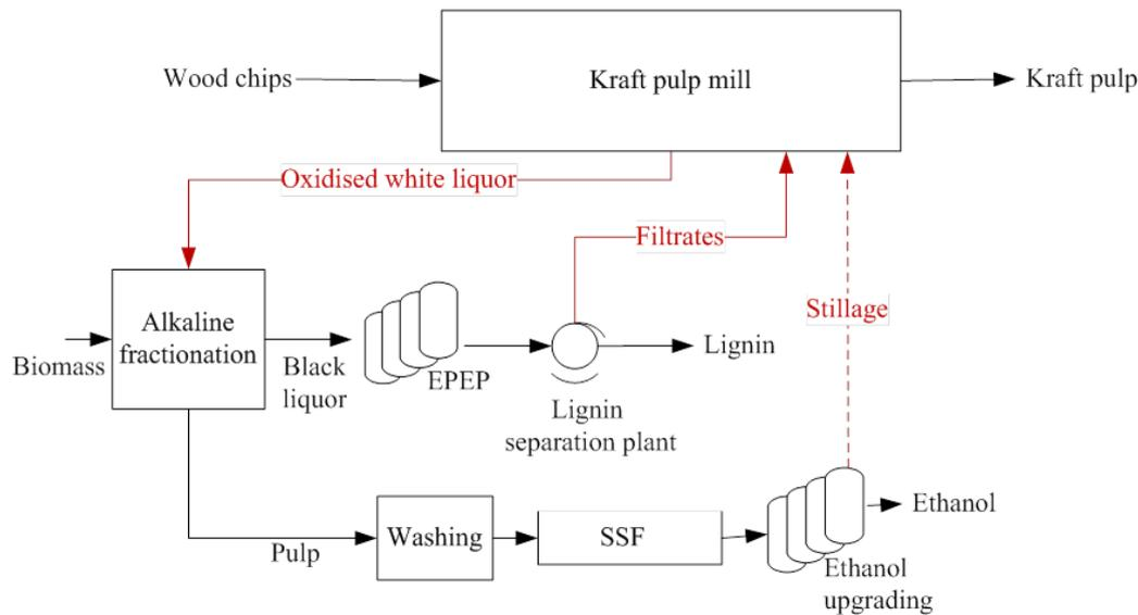
Figure 8 Alkaline-based high-solids ethanol process.
