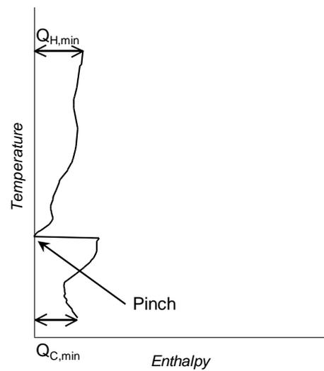
Figure A2: Example of shifted Composite Curves.
