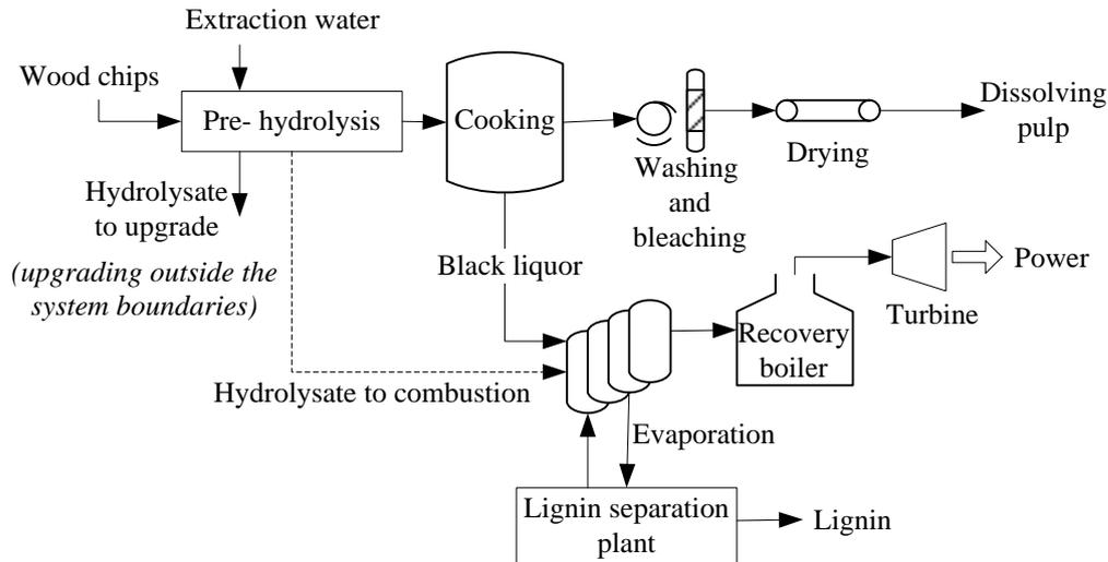
Figure 7 Kraft-based dissolving pulp process.
