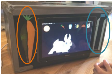
Figure 3: Second prototype with an app-solution and electronic interactions: feed (orange), giving water (blue), cleaning (at the back)
