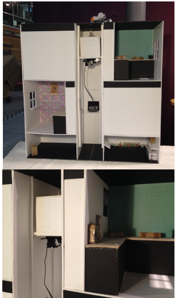
Figure 2. Display of our three stories house model in scale 1:5, The elevator delivers a package from the basement store to floor 3, right onto the kitchen sink.
