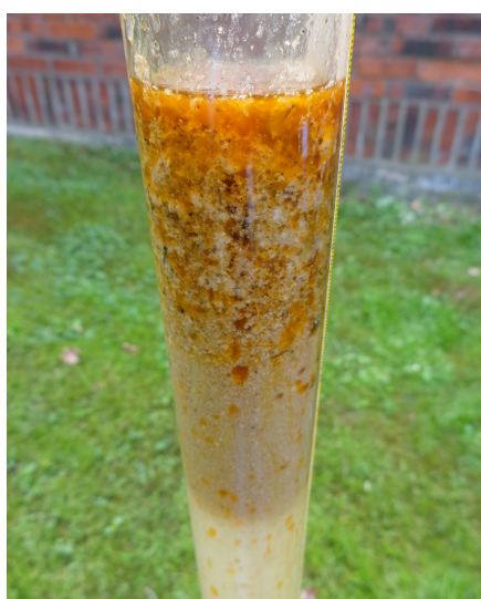
Figure 12: Sludge judge test showing the triphasic disposition on the grease cap at C1(2) at Restaurant Syster O Bror after 14 days of activity.
