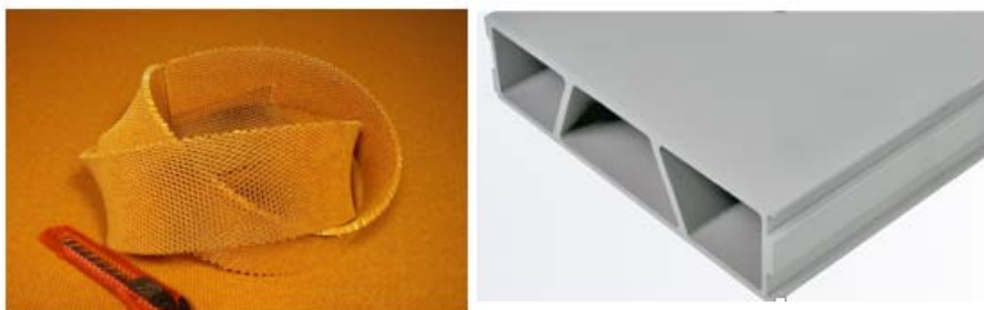
Figure 2.33 Honeycomb [31] and corrugated cores [14]
