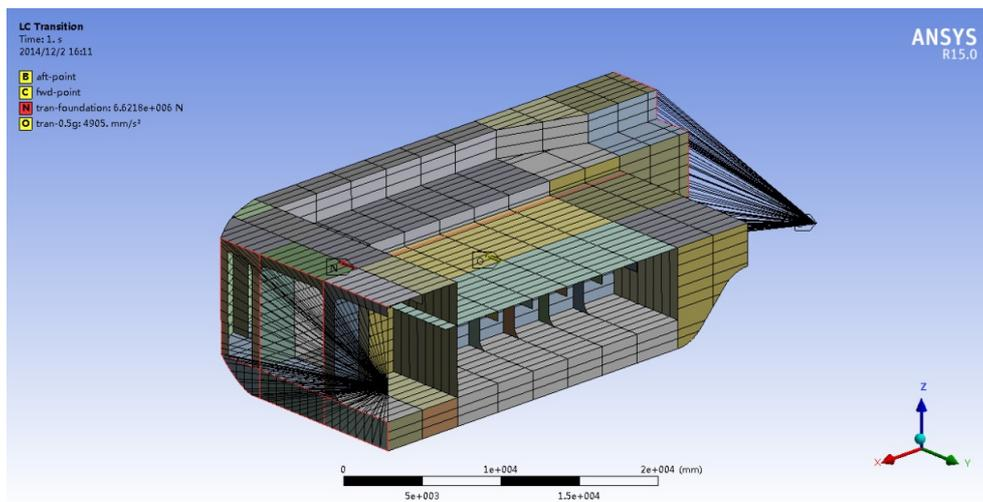
Figure 7.24. Transverse loading due to ship roll motion
