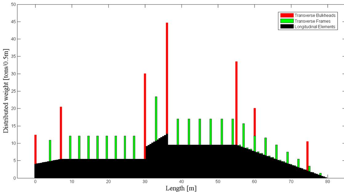
Figure 7.10. Steel weight distribution of bare hull
