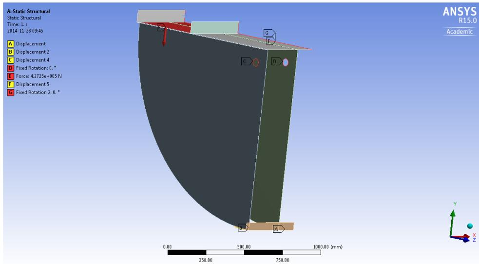
Figure 7.32. Boundary conditions on the retractable rail model
