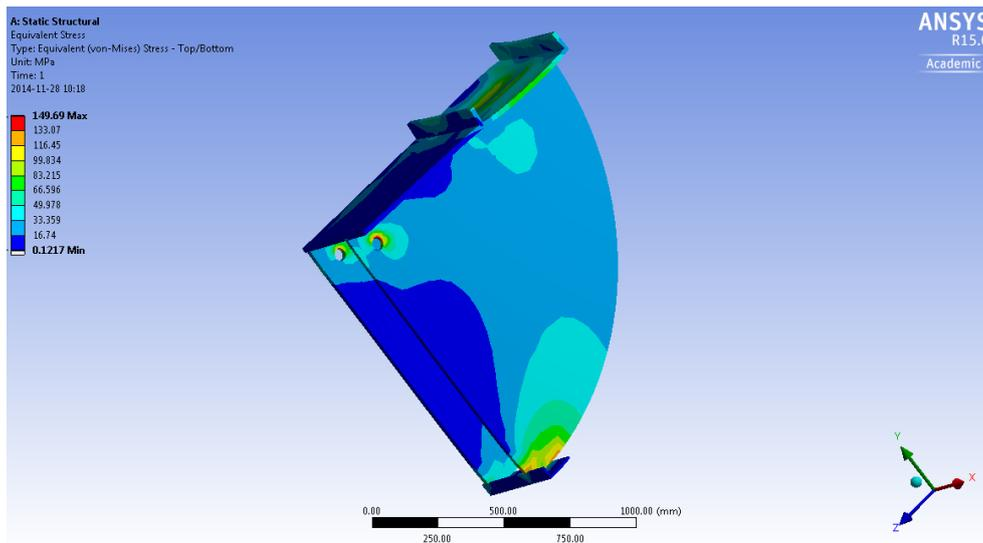
Figure 7.34 von Mises equivalent stress distribution of the retractable rails
