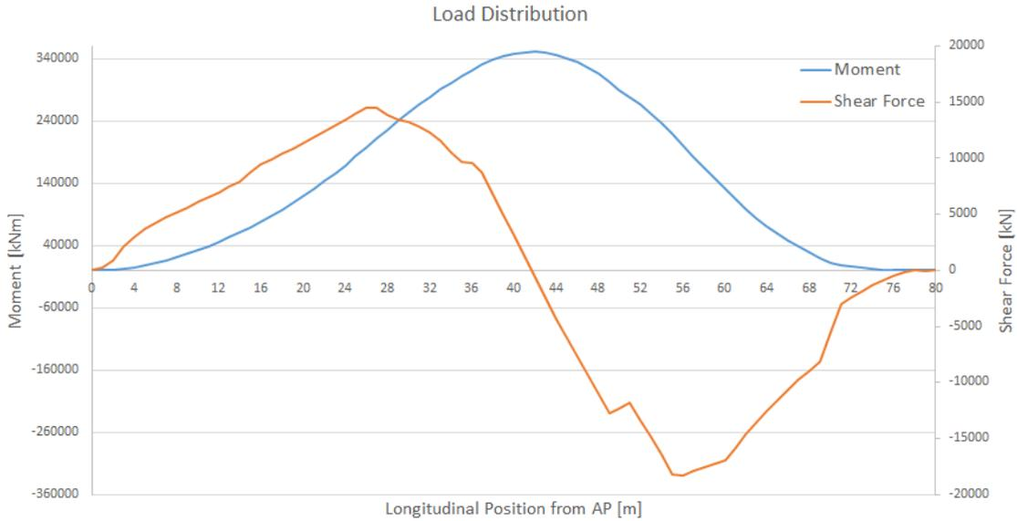
**Figure 7.3. Stillwater bending moment and shear force for largest single payload in offloading position.**
