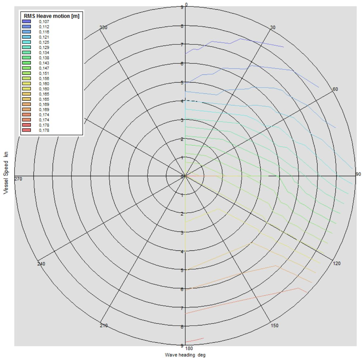
**Figure 5.6. Heave at the limiting operational sea state**
