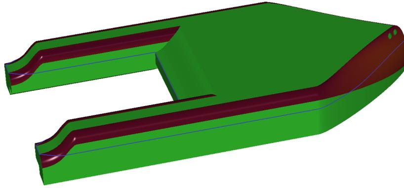
**Figure 5.6. Transverse curvature where transversely bended surfaces are blue or red other are green.**
