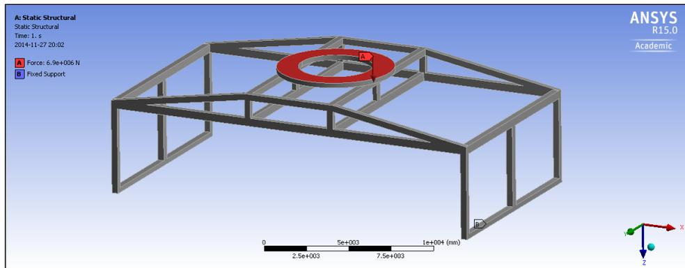
Figure 7.30. – Boundary conditions and loads on windmill fixture.
