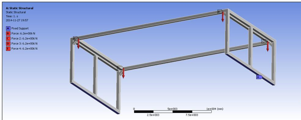
Figure 7.28. – Boundary conditions and loads on foundation fixture.
