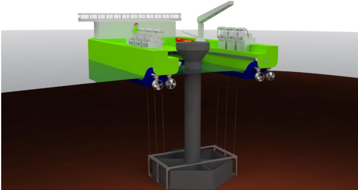
**Figure 3.6. Installation of foundation on the seabed.**
