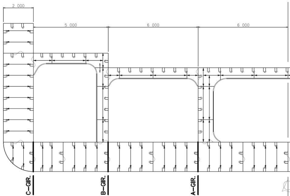
**Figure 7.9. Web frame and girder reference**
