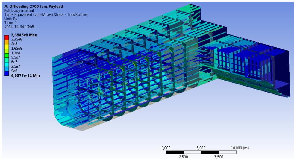
**Figure 7.13.** von-Mises Equivalent stress for the internal members on the global model.
