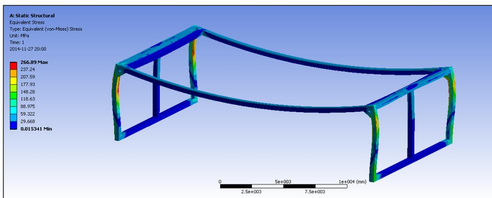
Figure 7.29. – Maximum von Mises stress of foundation fixture.
