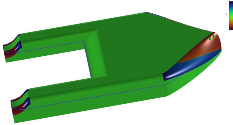
**Figure 5.4. Gaussian curvature where double bended surfaces are blue or red and single bended are coloured green**
