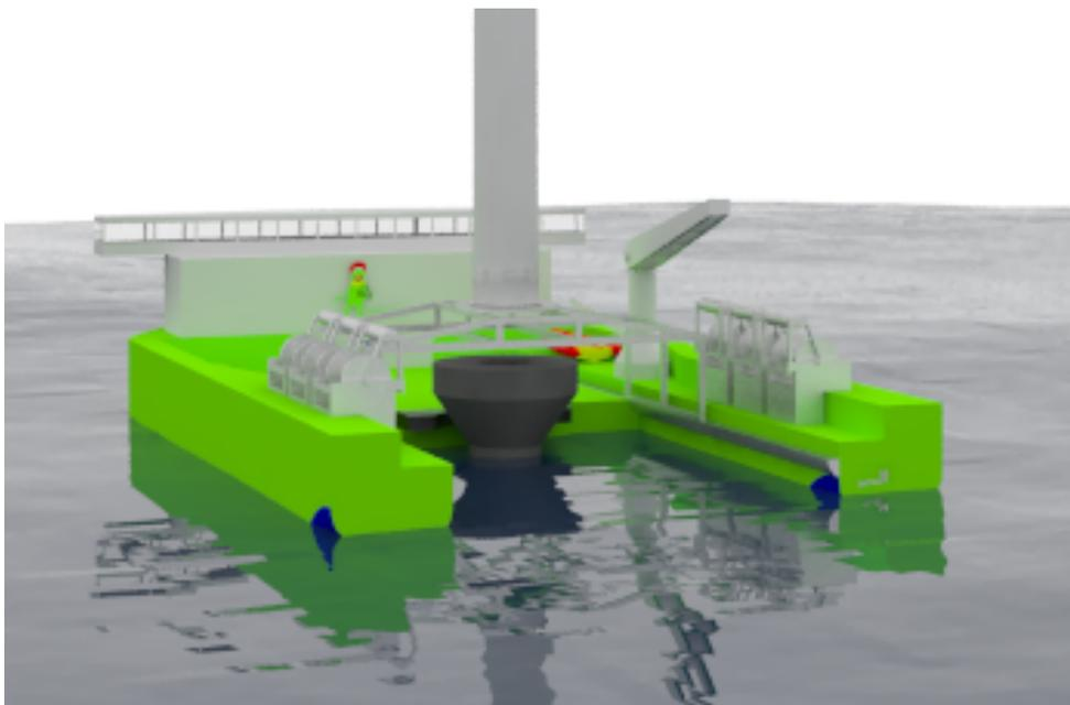
**Figure 3.7. Installation of a windmill on top of foundation.**
