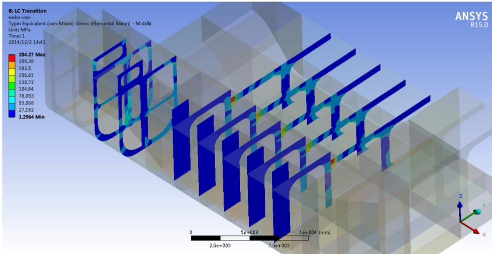
Figure 7.21. Transverse frame plates von Mises stress contour
