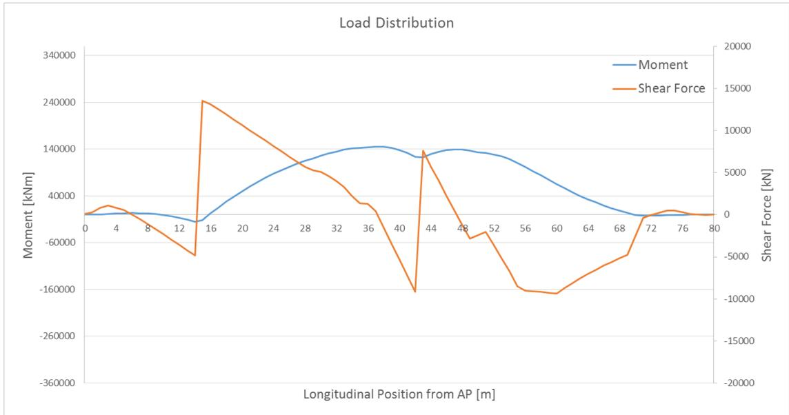
**Figure 7.5. Stillwater bending moment and shear force at largest total payload**
