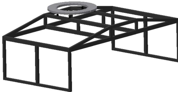
Figure 4.8. Principle sketch of the fixture to be used during operations with windmills.
