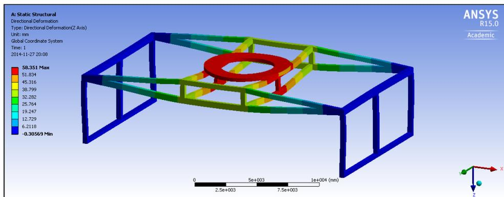
Figure 7.31. – Maximum deformation in z-direction for windmill fixture.
