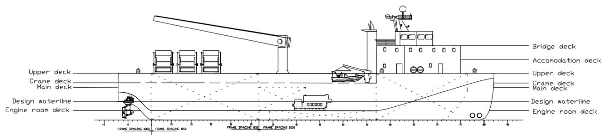
Figure 4.1. Side view of the vessel.
