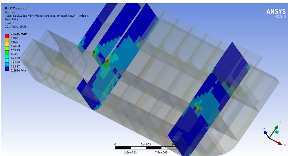
Figure 7.23. Transverse bulkhead plates von Mises stress contour
