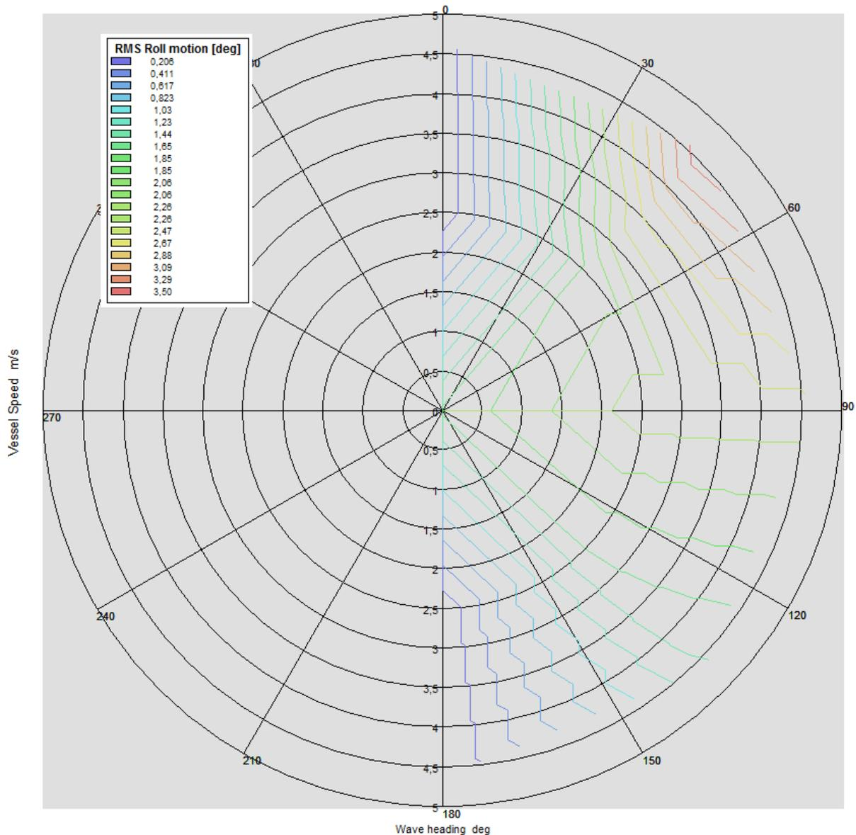
**Figure 5.7.** Roll motions at the limiting operational sea state
