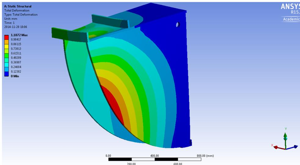
Figure 7.33. Total deformation of the retractable rails
