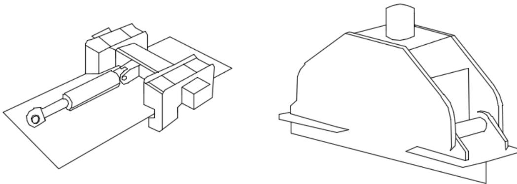
**Figure 4.10.** The left figure shows the principals of the push/pull unit and the right figure shows the principals of the skidshoe.
