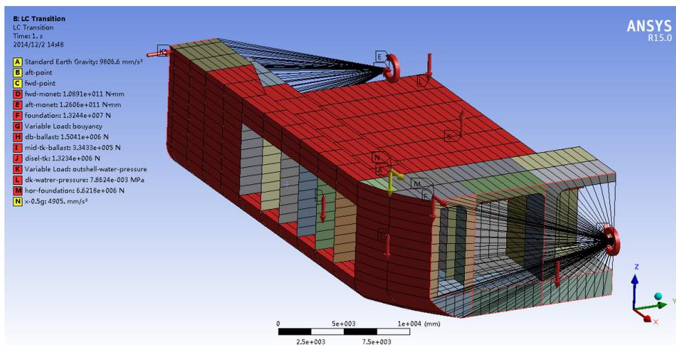
**Figure 7.19. The load implement under one foundation transition condition**
