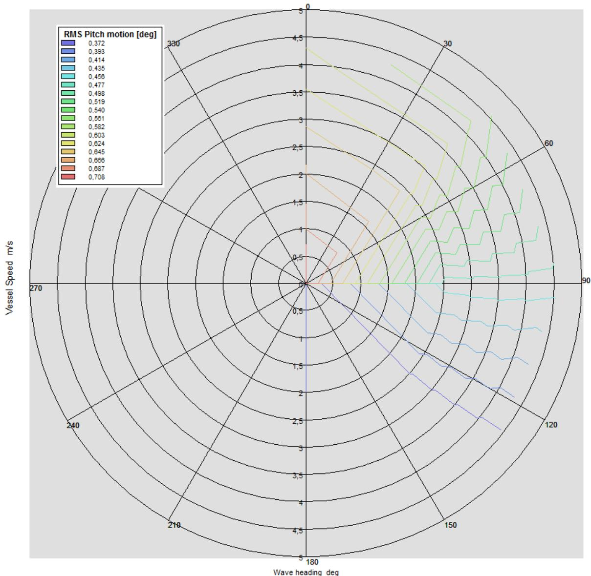
Figure 5.8. Pitch motions at the limiting operational sea state
