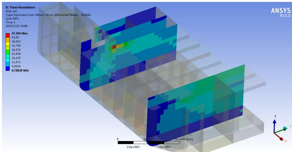
Figure 7.26. Transverse bulkhead von Mises stress contour under transverse loads
