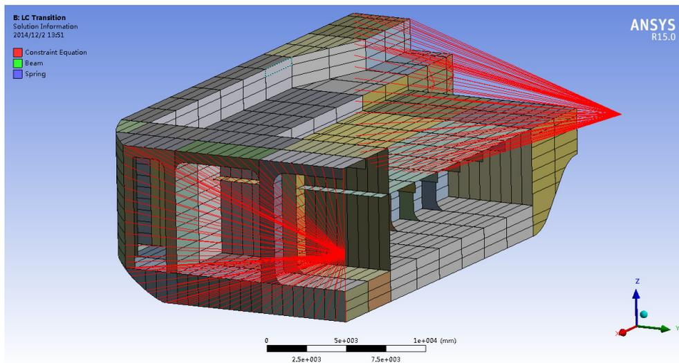
**Figure 7.18. MPC boundary condition setting at the ends of the model and mesh visualization (red lines represent connections between nodes and the remote points)**
