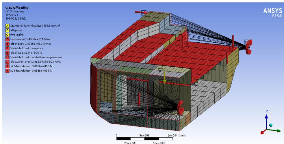
**Figure 7.20. The load implement one foundation offloading condition**
