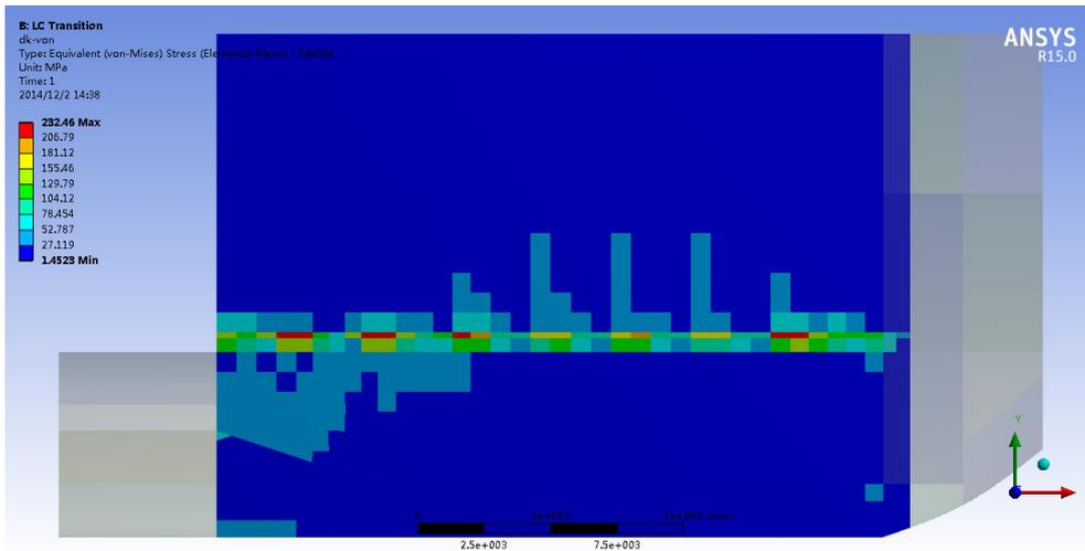
Figure 7.22. Deck plates von Mises stress contour in transition load condition
