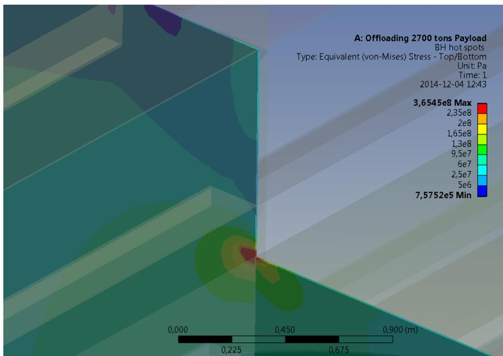
**Figure 7.14.** Stress concentration in bulkhead at catamaran/transition zone interface (upper corner)
