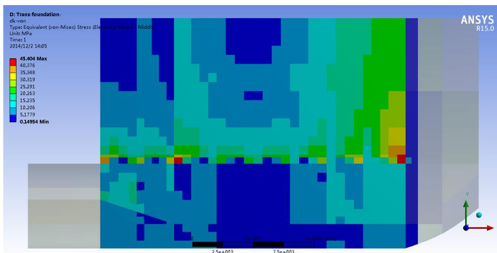
Figure 7.25. Deck von Mises stress contour under transverse loads
