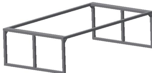
**Figure 4.7. Principle sketch of the fixture to be used during operations with foundations.**
