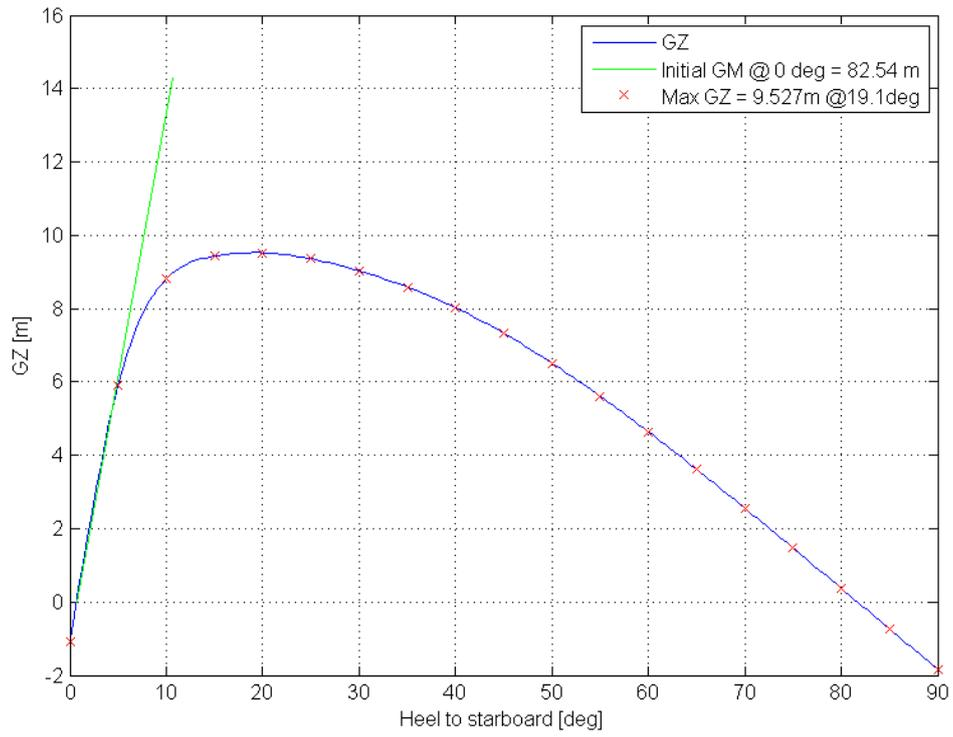
**Figure 5.5. GZ curve for lightship condition with Max value at 9.527m at 19.1 deg. including initial GM= 82.54 m at 0.0deg.**
