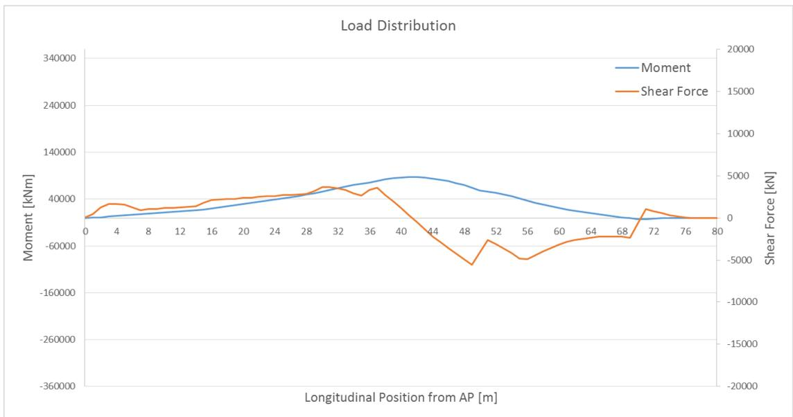
**Figure 7.6. Stillwater bending moment and shear force at ballast condition**
