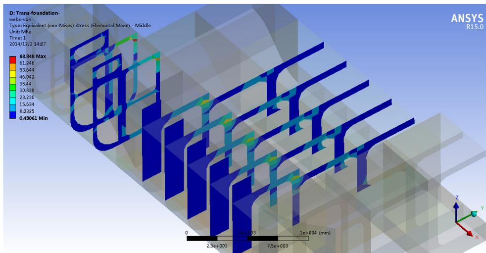
Figure 7.27. Web frame von Mises stress contour under transverse loads
