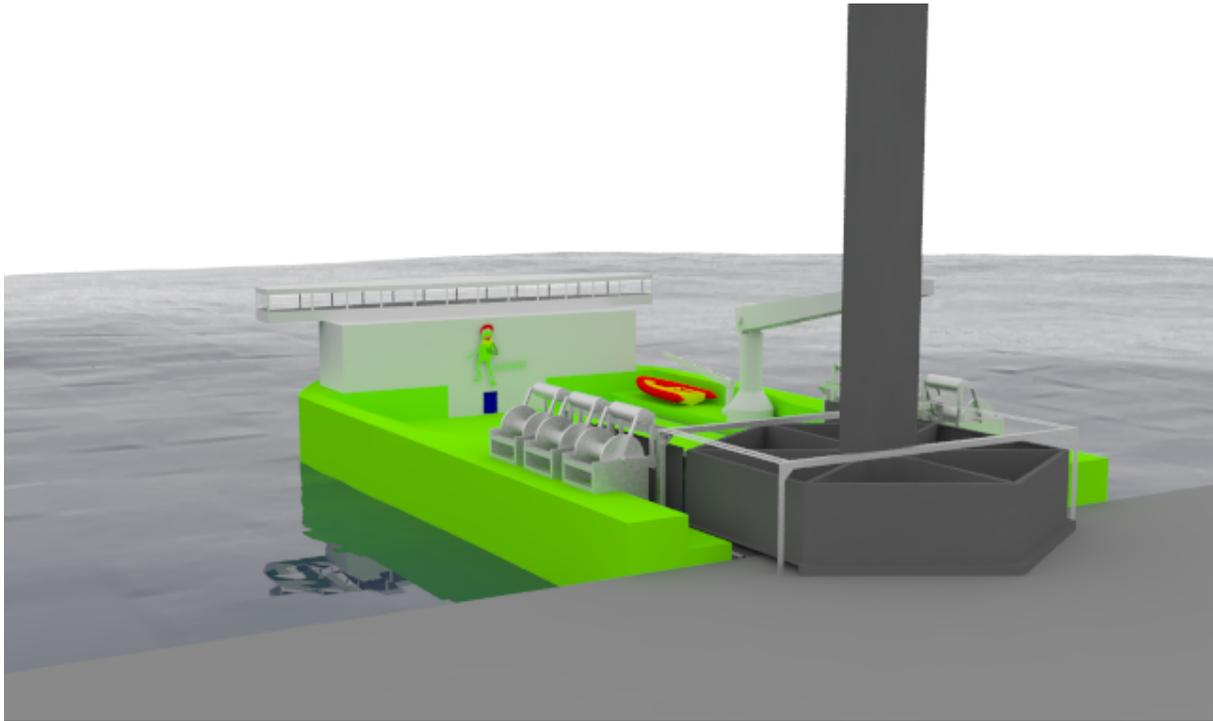
**Figure 3.4. Loading of foundation in port.**
