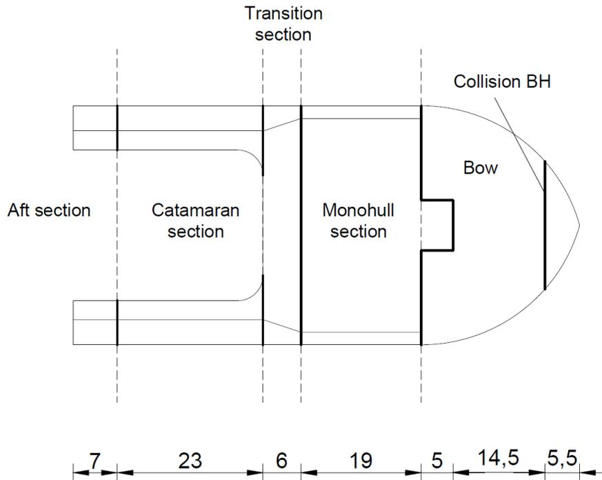
**Figure 7.1. Longitudinal division of hull girder sections**
