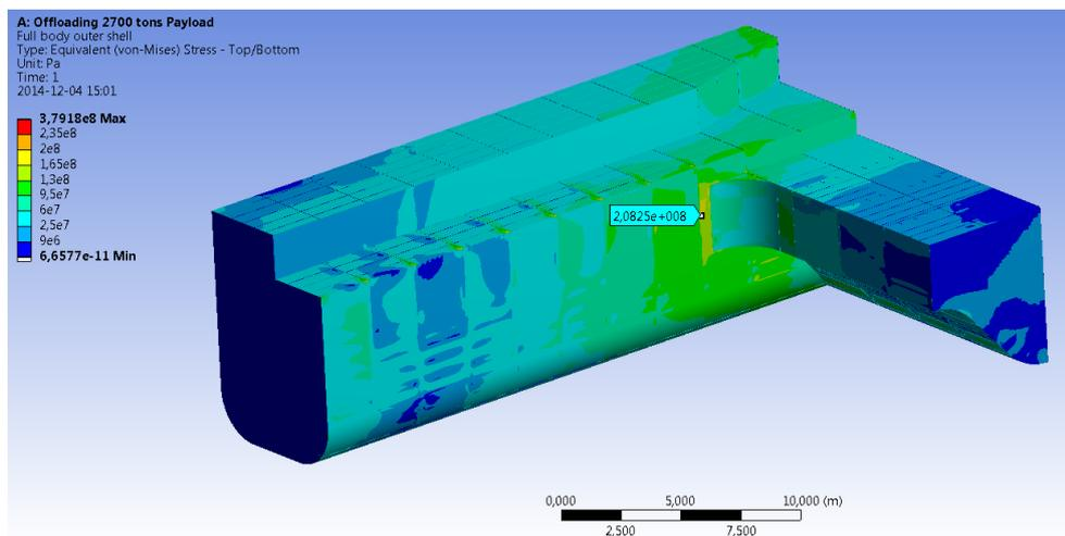
Figure 7.12. von-Mises Equivalent stress for the outer shell on the global model (inner side and deck).
