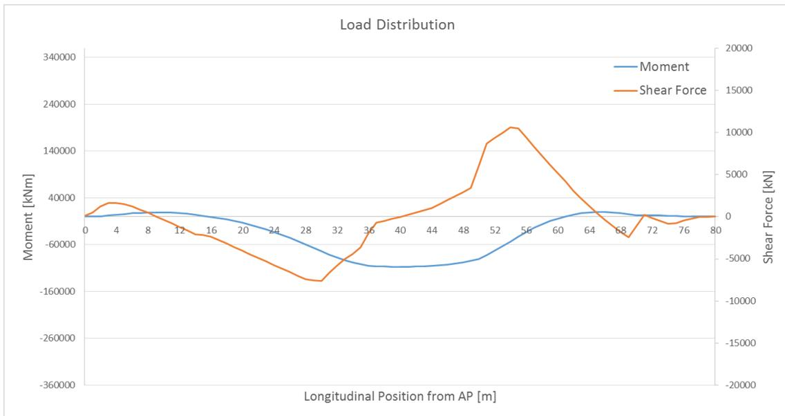
**Figure 7.4. Stillwater bending moment and shear force for largest single payload in transit position.**
