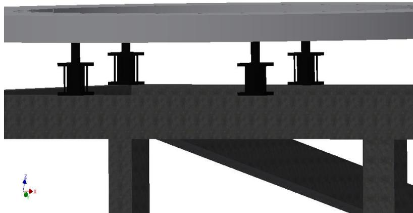
Figure 4.9. Principle sketch of the jack-ups on the windmill fixture.
