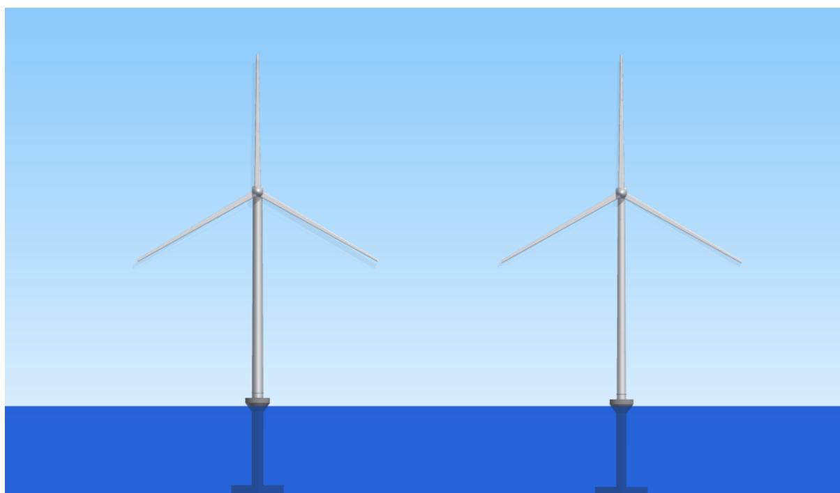
Figure 2.1. Windmill mounted on gravity foundation
