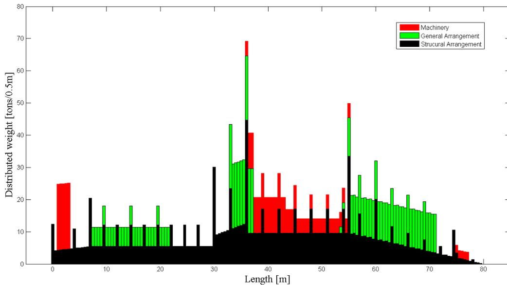
Figure 4.12. Light ship estimation of Kermit
