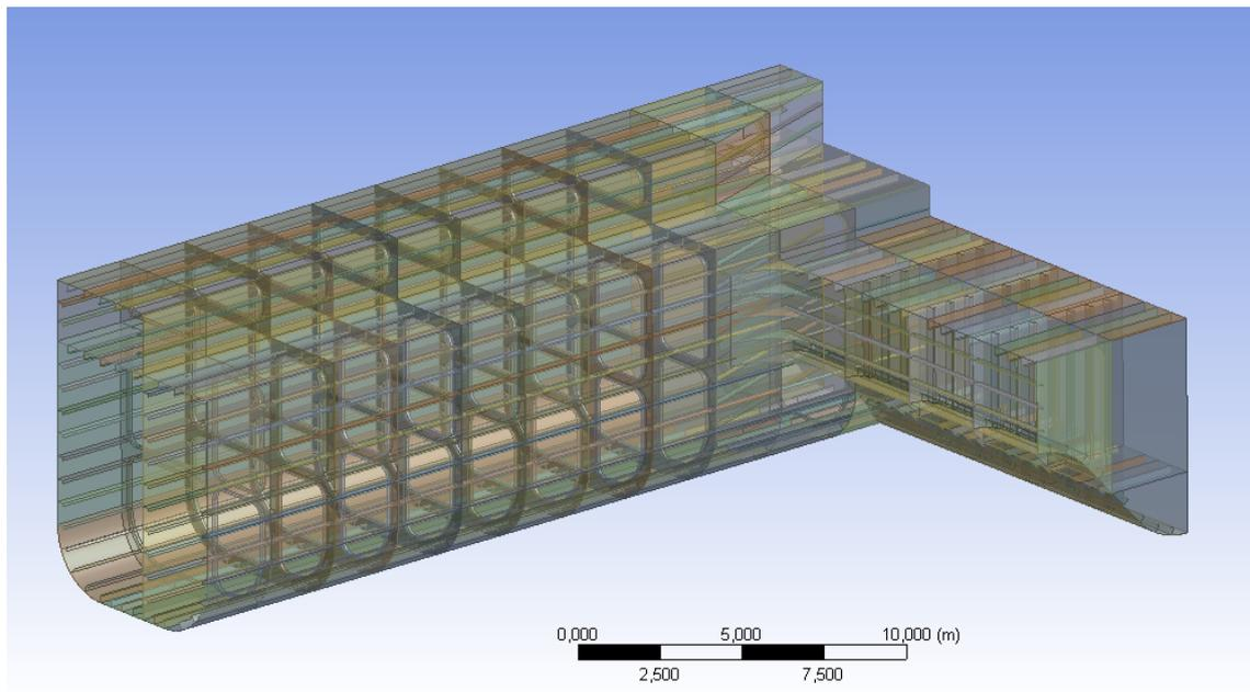
**Figure 7.11. Geometry representation of the evaluated FE-model**
