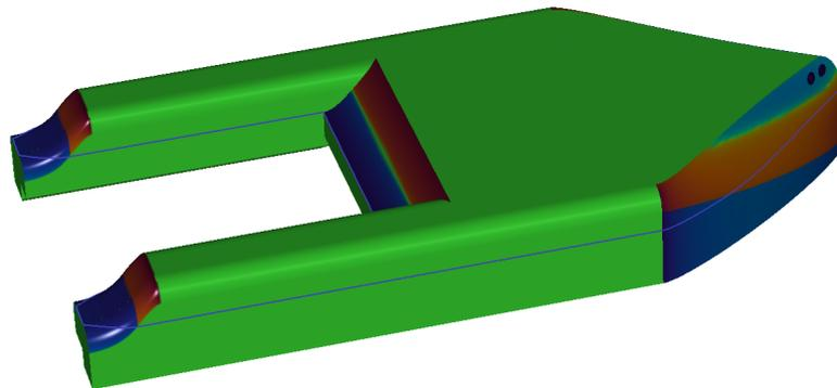
**Figure 5.5. Longitudinal curvature where longitudinally bended surfaces are blue or red other are green.**
