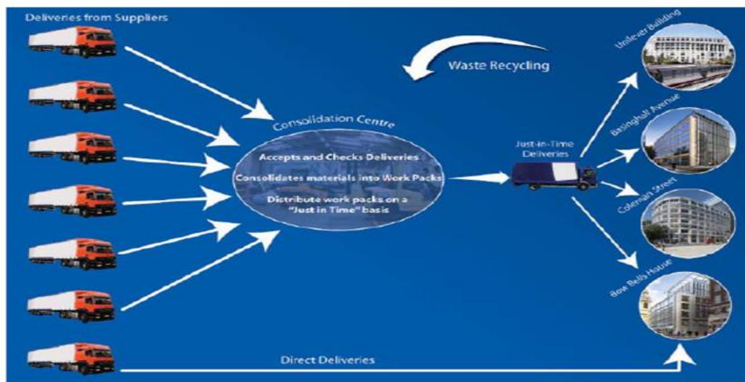
Overview of the LCCC operation to the four construction sites (Stanhope and Wilson James 2008),
