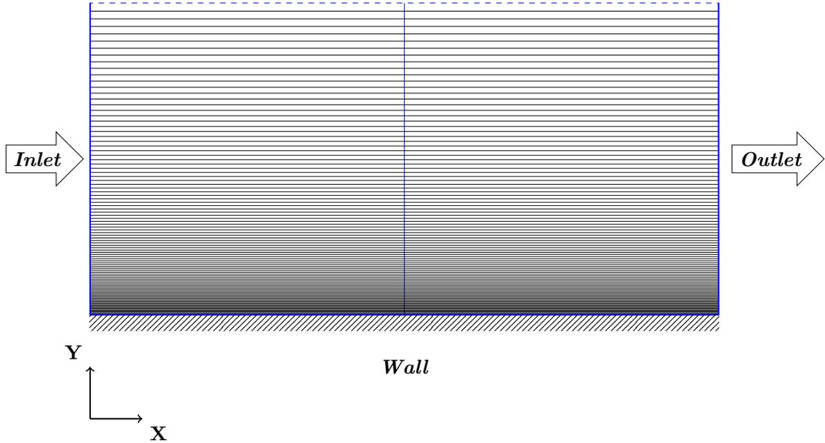
The channel mesh is generated by the 'blockMesh' utility. There are a total of  $2 * 100 * 1$  cells. Apart from the four patches in the figure above ('inlet', 'outlet', 'wall', 'symmetryPlane'), the z-faces are named as 'frontAndBack' and are classified as 'empty' patches.
