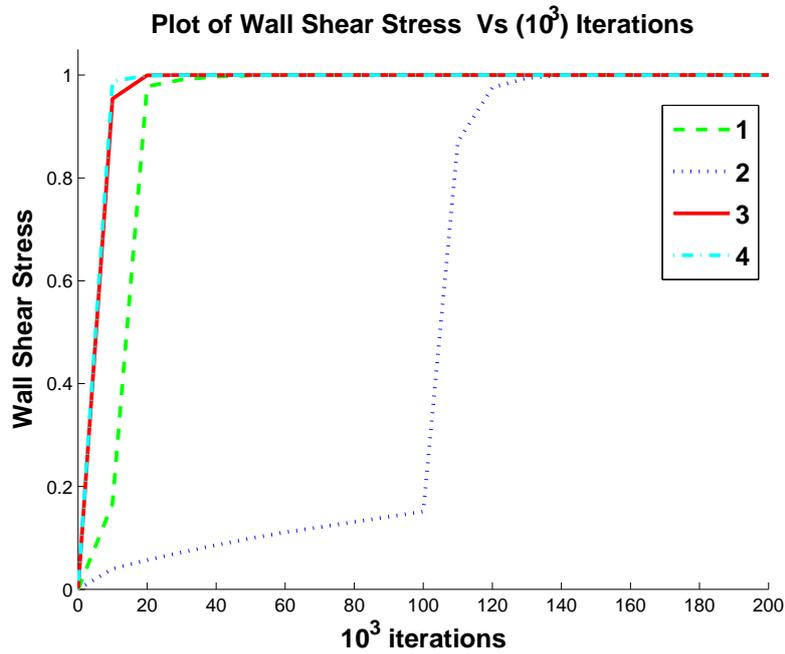
**Figure 6.8:** Wall Shear Stress vs  $(10^3)$  iterations at  $Re_\tau = 395$  [1- Chien  $k \epsilon$ , 2- EARSM + Chien  $k \epsilon$ , 3-  $\phi$ -f, 4- EARSM +  $k \omega$  BSL]
