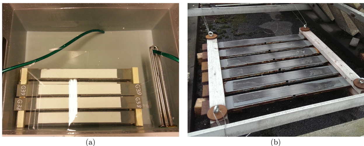
Figure 5.3. Exposure of DLS specimens: (a) heated-water tank, (b) outdoor conditions.
