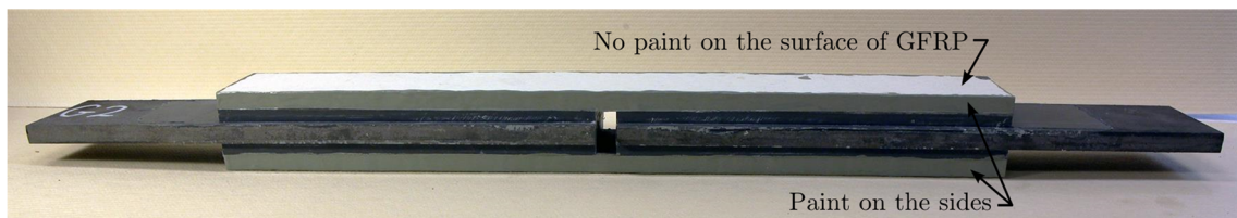
(b) DLS with side-painted GFRP adherends
