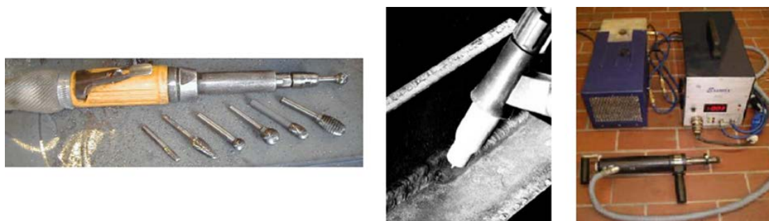
Figure 3. Burr grinding (left), TIG dressing (middle) and UIT (right) tools [4][11].
