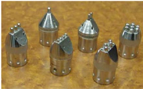
Figure 6. Example of indenter size and configurations. Photo courtesy of Integrity Testing Laboratory (ITL) and Structural Integrity Technologies Inc. (SINTEC) [10].
