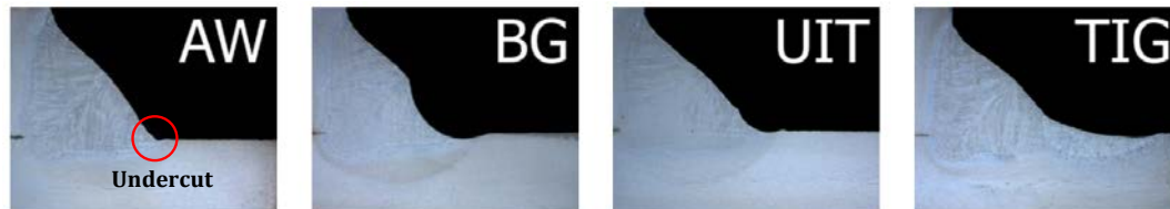
Figure 2. The as-welded (AW) weld profile with the undercut defect and the weld profiles after treatment with burr grinding, ultrasonic impact treatment and TIG dressing, respectively. Adapted from [4].
