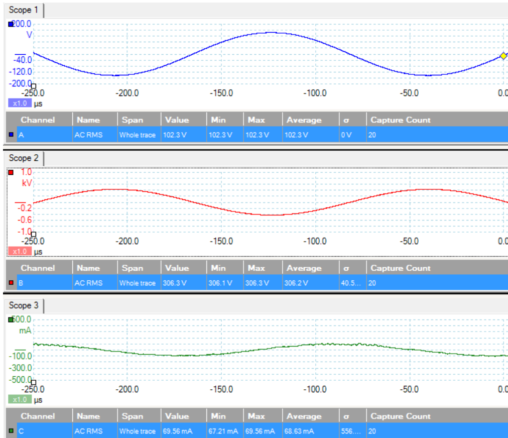
Figure 5-28: Picoscope’s on screen recordings for the Nano transformer; 100V sinusoidal at secondary, 300V at primary and 70 mA supplied current.
