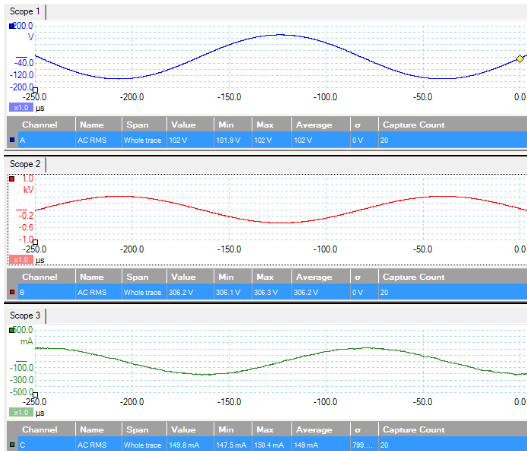
Figure 5-27: Picoscope's on screen recordings for the Ferrite transformer; 100V sinusoidal at secondary, 300V at primary and 150 mA supplied current.
