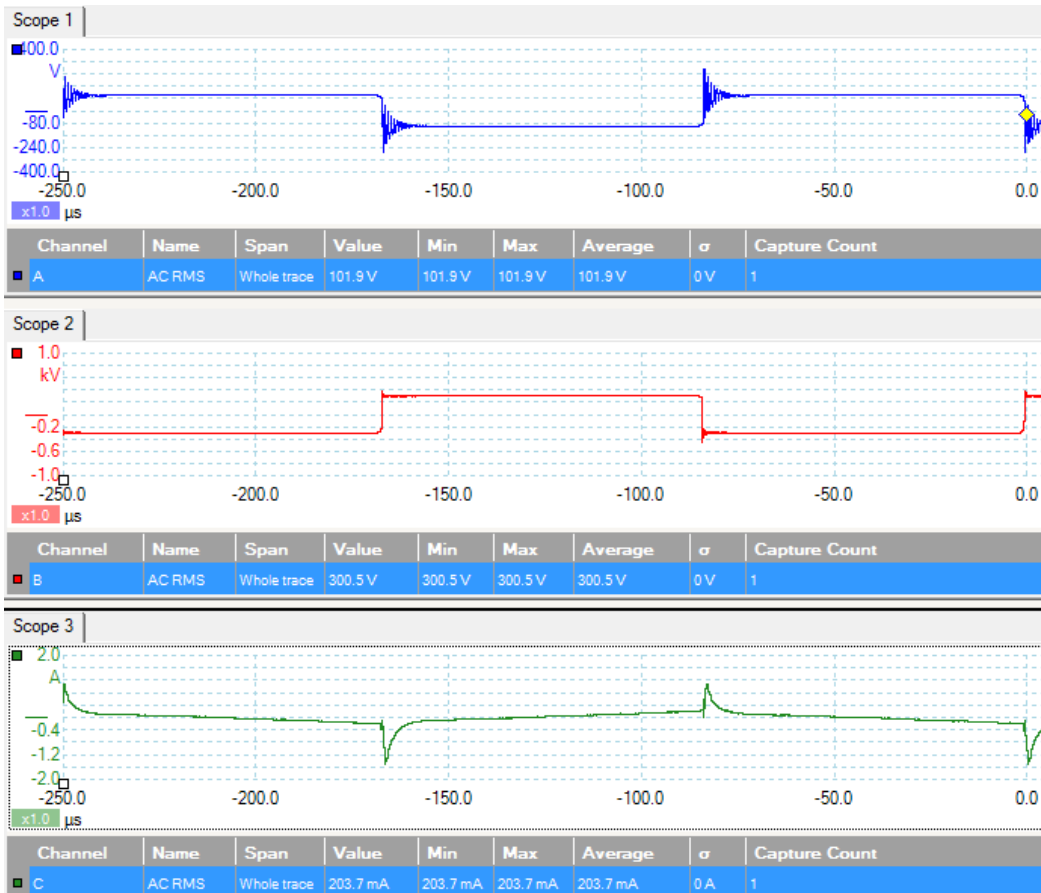
Figure 5-24: Picoscope's on screen recordings for the Ferrite transformer; 100 V at secondary, 300 V at primary and 204 mA supplied current.
