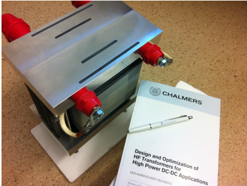
Title photo: The Nanocrystalline transformer without heatsinks.
