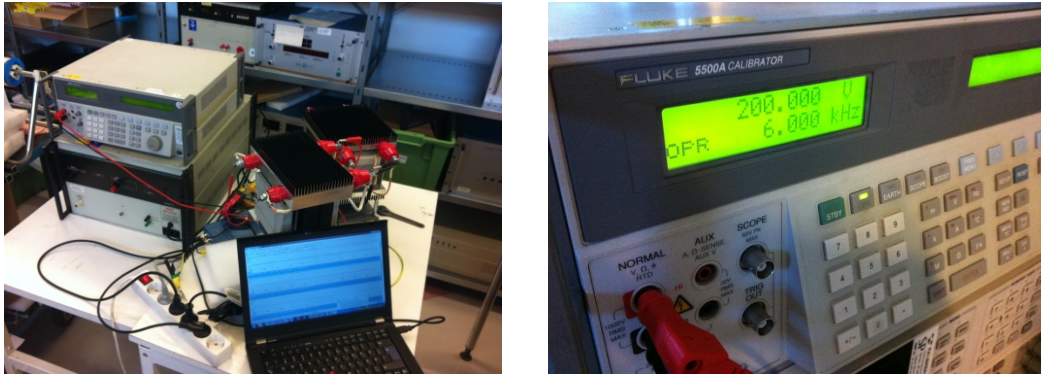
Figure 5-26: No-load test circuit (a) on transformers at 6 kHz with sinusoidal voltage performed using a Fluke 5500 calibrator as a voltage source (b).
