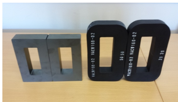
Figure 3-1: One Ferrite core stack (left) compared with one Nanocrystalline core stack (right).
