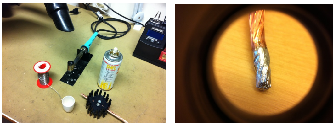
Figure 3-12: Soldering the litz wires.
