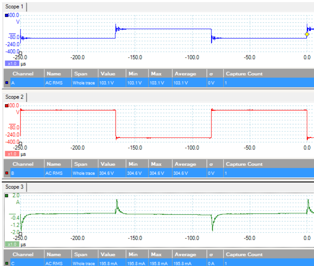
Figure 5-25: Picoscope's on screen recordings for the Nano transformer; 100 V at secondary, 300 V at primary and 196 mA supplied current.
