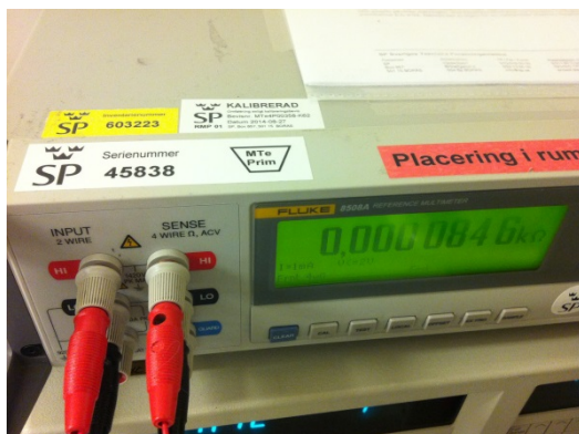
Figure 5-2: LV Resistance measurement using a reference multimeter and the 4 wire method.
