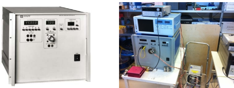
Figure 5-29: The load loss test on transformers using a Clarke-Hess, 8100, Trans-conductance amplifier.
