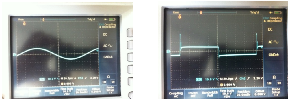
Figure 5-19: Sinusoidal and square waves at the maximum applicable voltage by Fluke 5205.
