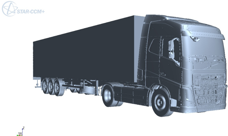
Figure 2.1: CAD models of a FH16 H2 tractor with semi-trailer.
