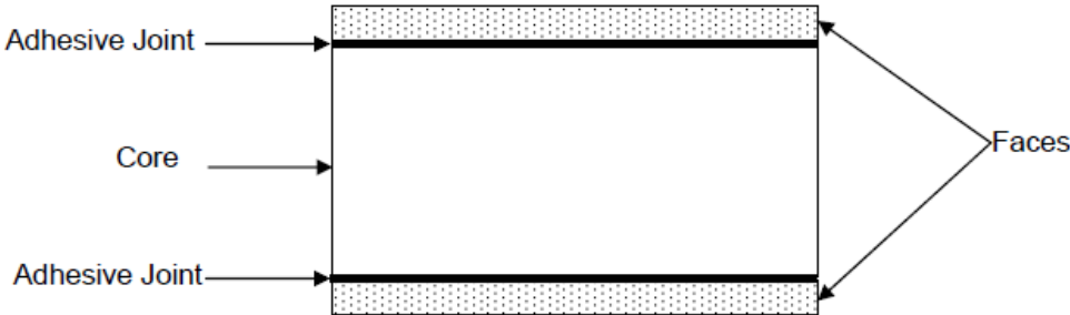
Figure 2.30 Principal illustration of a sandwich element [29]
