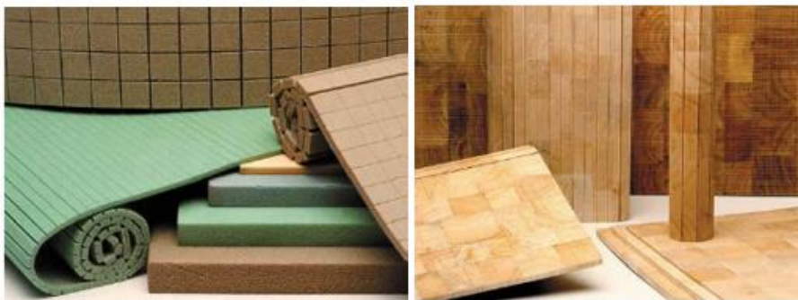
Figure 2.32 Foam and balsa wood cores [30]
