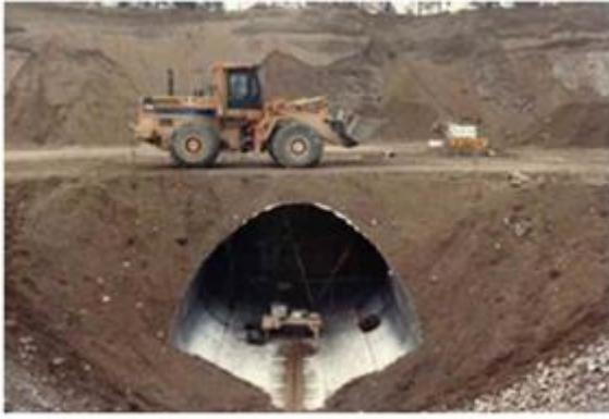
Figure 2.2 The field test of pipe arch culvert in Sweden in 1987-1990 [3]
