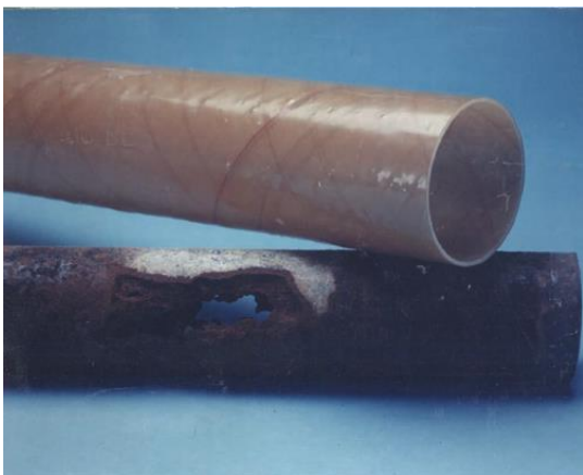
Figure 2.25 FRP pipe versus steel pipe for water applications [17]
